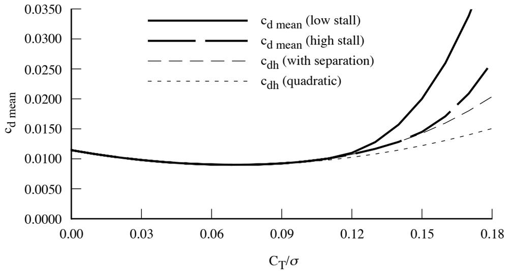
Figure 11-8. Mean drag coefficient for rotor in hover.
