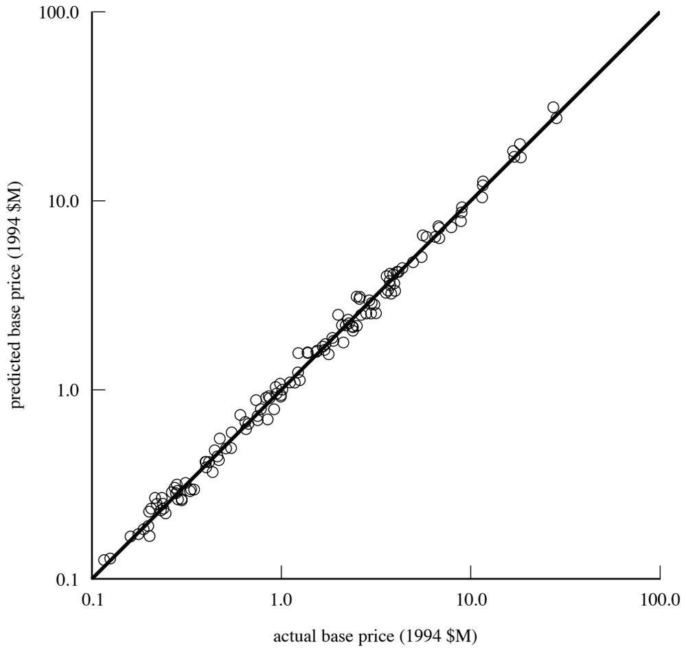
Figure 6-2. Statistical estimation of rotorcraft flyaway cost (\$M).
