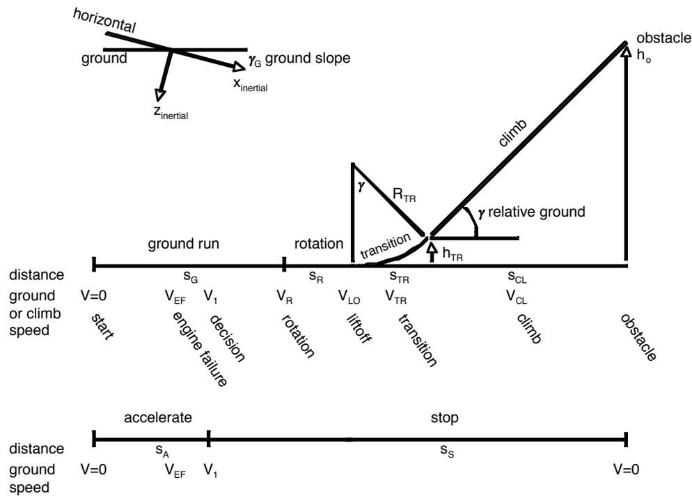
Figure 4-1. Takeoff distance and accelerate-stop distance elements.
