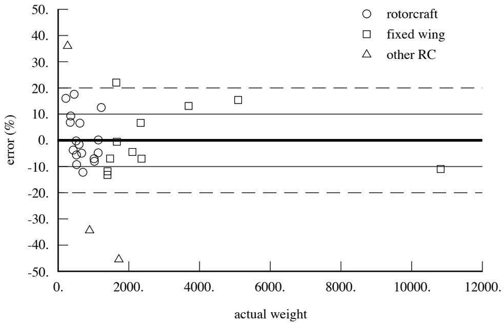
Figure 19-11. Alighting gear group, landing gear weight (AFDD82).
