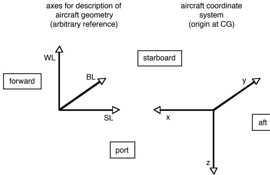
Figure 7-1. Aircraft geometry.
