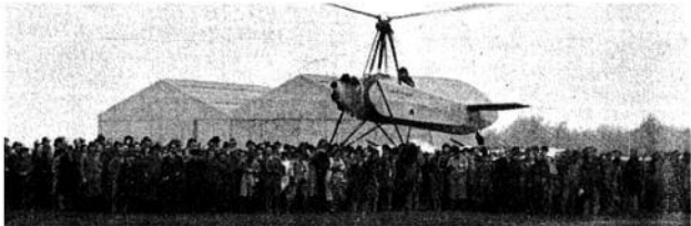
Fig. 2-37. Raoul Hafner publicly demonstrated the prototype of our modern swashplate control system with his A.R. III on May 9, 1937 [74].
