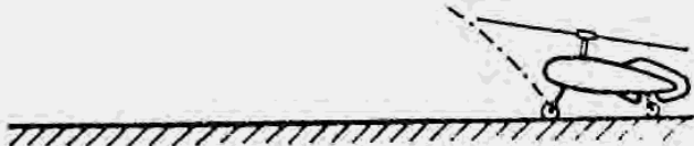
FIGURE 16. Path of machine during direct take-off.
