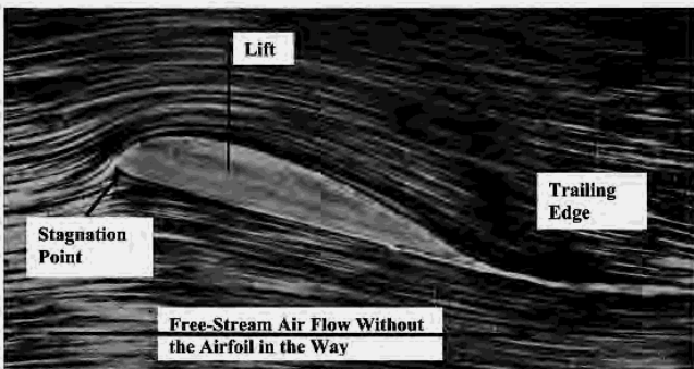
Fig. B-1. Air flow around a cambered airfoil set at positive angle of attack.
