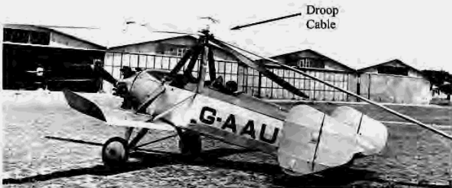
Fig. 2-73. Cierva C.19 Mk. III showing “droop” and lead-lag cables [7].
