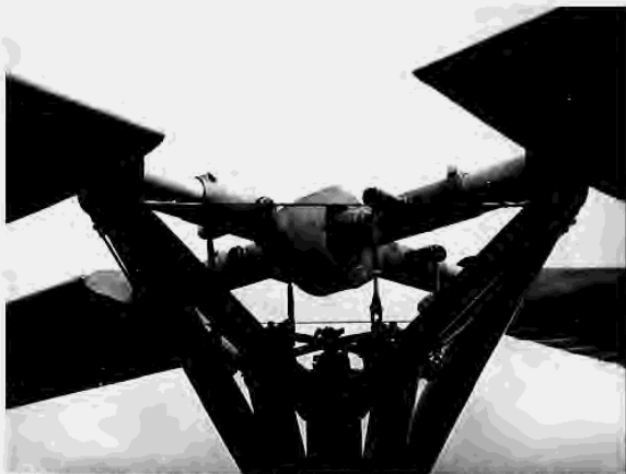
Fig. 2-35. The Wilford rotor system had neither flapping nor lead-lag hinges. Instead, blade feathering followed Eq. (2.57) to zero the rolling moment (photo courtesy of Wayne Wiesner).
