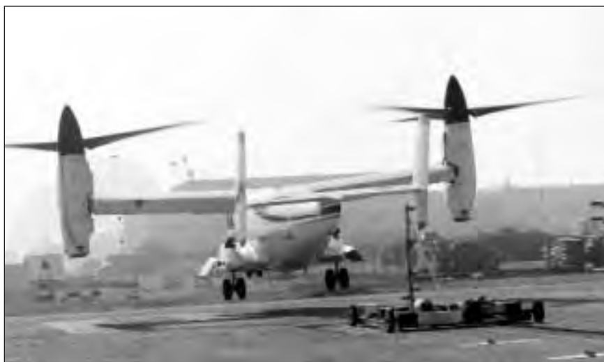
Figure 50. XV-15 hovering in-ground-effect during 1984 performance and downwash test. (Ames Photograph AC81-0165-152)
