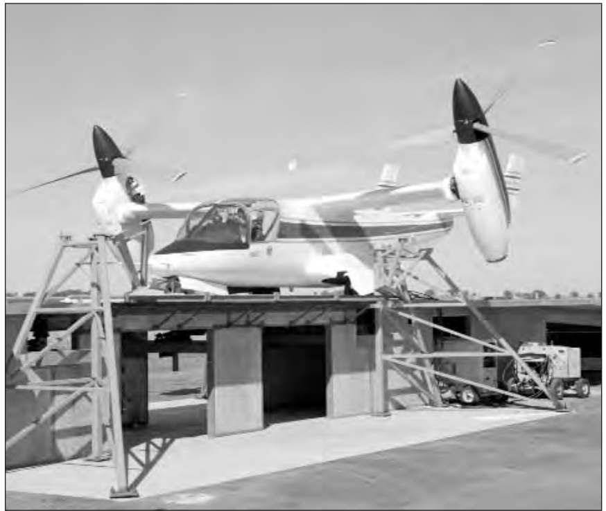
Figure 43. Bell XV-15 ground tiedown facility. (Ames Photograph AC76-1518-115)
