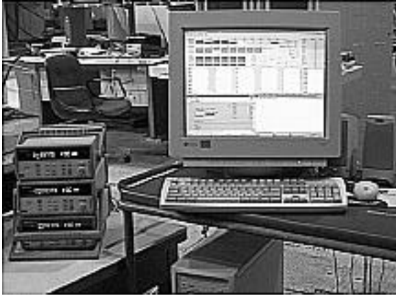
Figure 13: HP 34970A data acquisition / switch units and data acquisition computer
