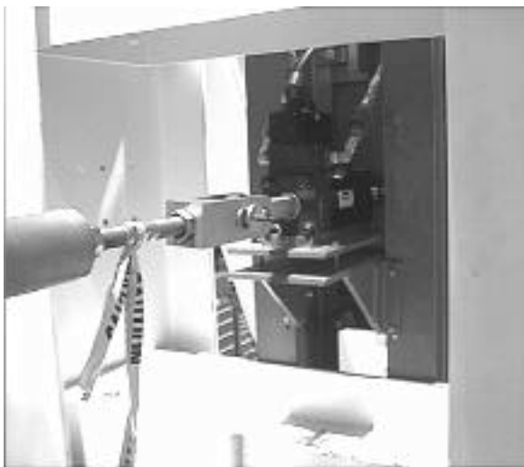
b. Calibration rig end, showing actuator
