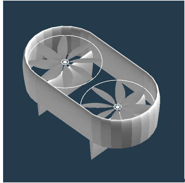
Figure 39. Nacelle control vanes in Oval ducts: (a) side ('cutaway') view and (b) isometric view
