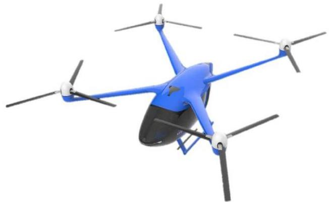
**Figure 3. Quadrotor Concept Vehicle, Ref. 2**
