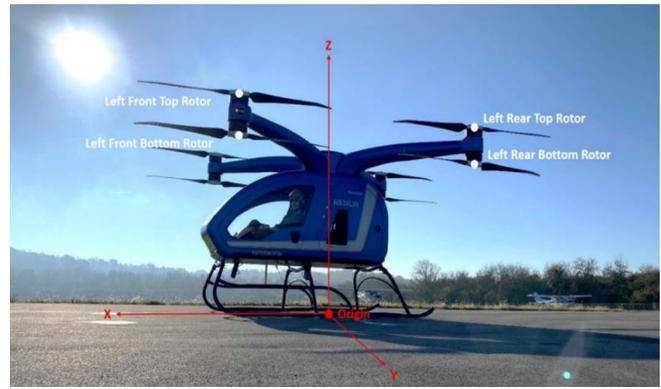
**Figure 2. Example Coaxial Quadrotor Vehicle, Ref. 17**
