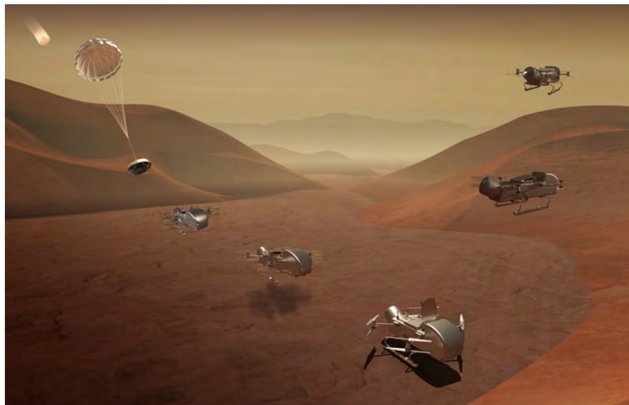
Fig. 2 An artist's impression of Dragonfly's concept of operations consisting of entry, descent, and first landing; surface operations; and atmospheric flight on Titan. Image courtesy of NASA/Johns Hopkins APL/Steve Gribben/Magda Saina ( https://dragonfly.jhuapl.edu/Gallery/ ).
