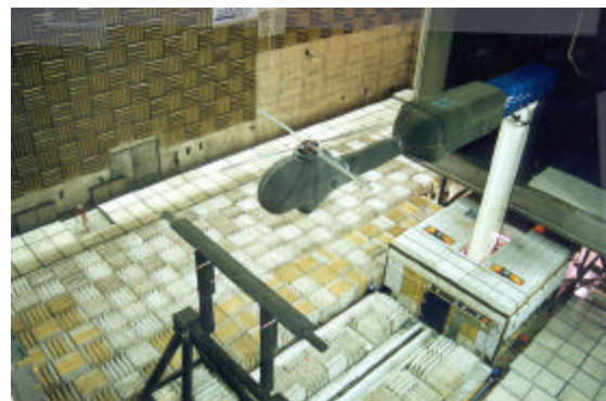
Fig. 1 BO-105 model rotor in the DNW
