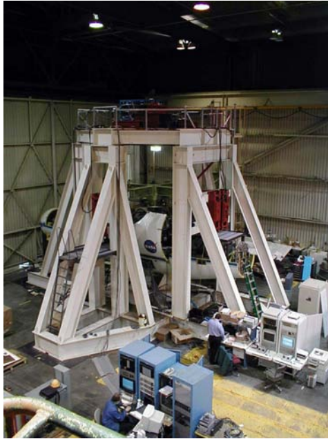
Figure 5.17. Dynamic calibration setup for Large-Scale Rotor Test Apparatus (LRTA).
