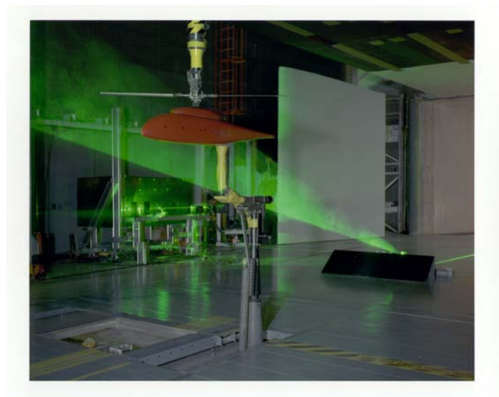
Figure 5.7. Doppler global velocimetry in use at the Langley 14- by 22-Foot Subsonic Wind Tunnel.
