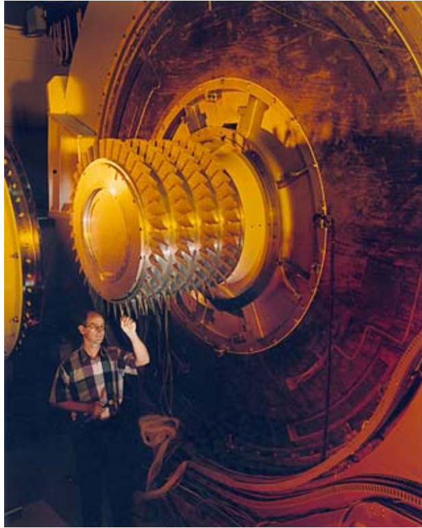
a) Large Low Speed Compressor facility
