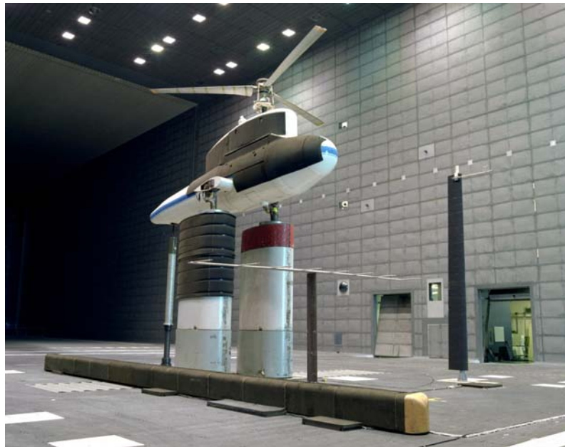
a) XV-15 rotor with higher-harmonic control installed on the Rotor Test Apparatus in the 80- by 120-Ft Wind Tunnel
