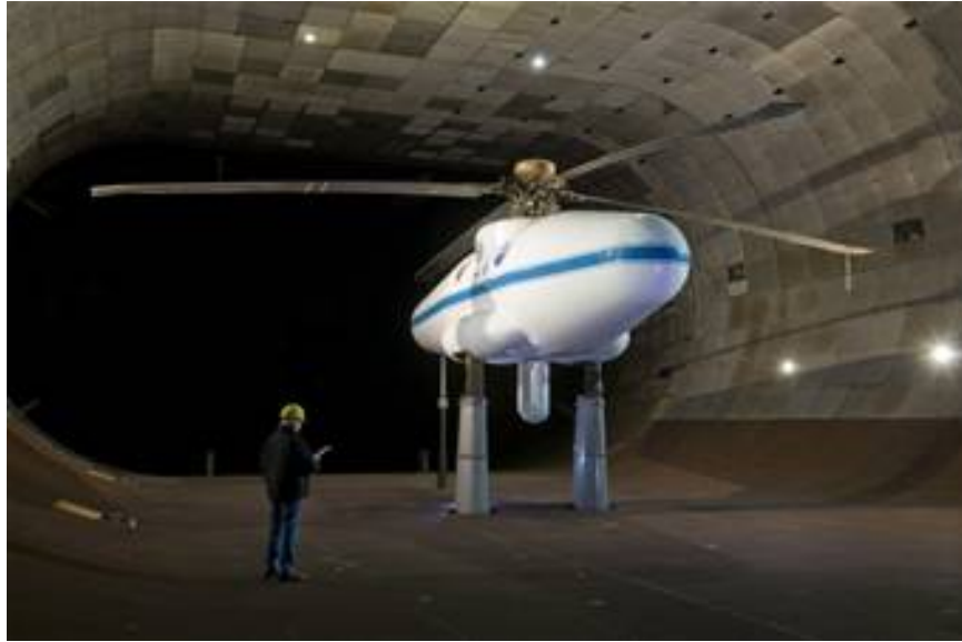
b) UH-60 rotor with individual blade control installed on the Large Rotor Test Apparatus in the 40- by 80-Ft Wind Tunnel
