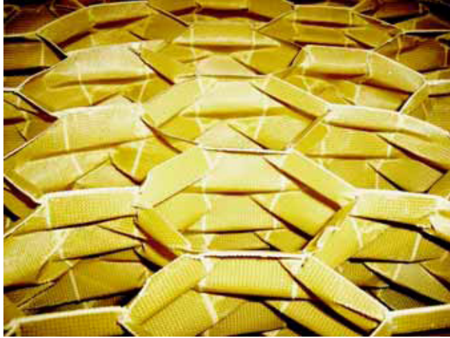
Figure 8.19. Postcrush photograph of a deployable honeycomb made of Kevlar.
