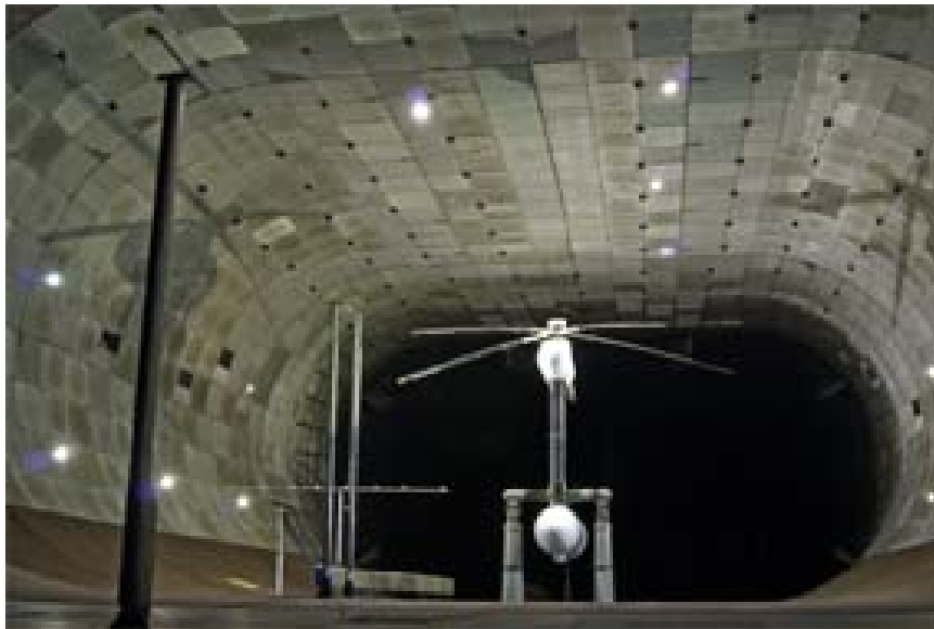
c) Boeing SMART rotor with active flaps installed in the 40- by 80-Ft Wind Tunnel
