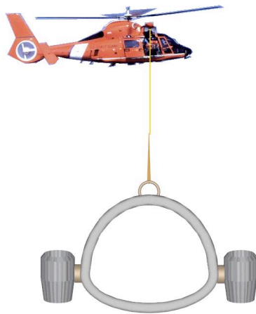
Fig. 19. "Vectored" Rescue Hoist Module Suspended from Helicopter
