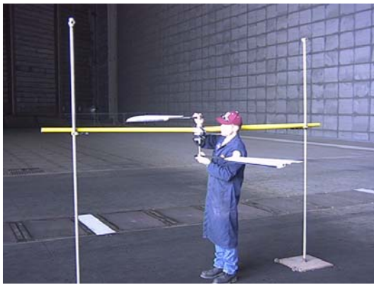
Fig. 12 – Mars Coaxial Rotor Hover Test; (a) conceptual sketch; (b) early stages of test hardware development
