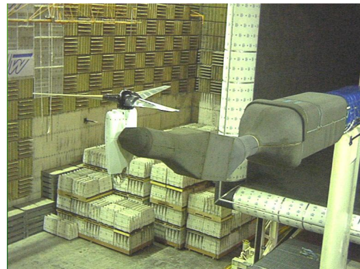
Fig. 1. TRAM Isolated Rotor Configuration in the Duits-Nederlandse Windtunnel (DNW) in The Netherlands
