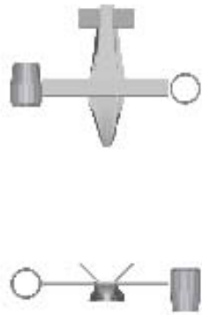
Fig. 11 – Orthogonal View of a Titan VTOL Concept
