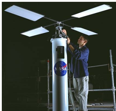
Fig. 3 – Baseline Proof-of-Concept Mars Rotor and Hover Test Stand
