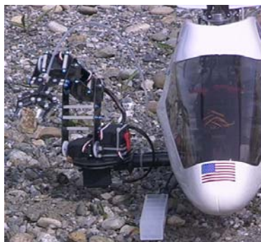
Fig. 9 – Rock/Soil Sampling from a Robotic Helicopter
