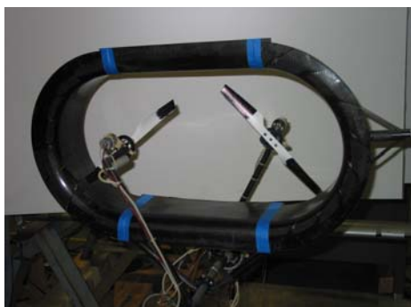
Fig. 21 – Elliptical Ducted Fan Test Installation
