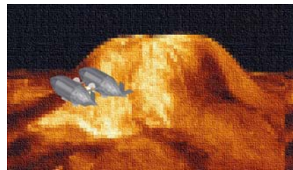
Fig. 25 -- A Notional Venusian Hybrid Airship with Twin Hulls and Tandem Tilting Propellers and Wings
