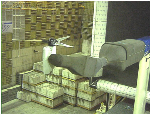
Fig. 1 -- Isolated rotor TRAM configuration (Installed in DNW Open-Jet Test Section)
