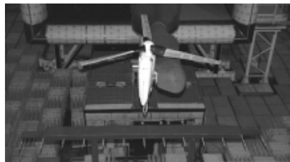
Figure 1. Isolated TRAM installed in DNW-LLF (view from above and upstream of model; microphone array in foreground).
