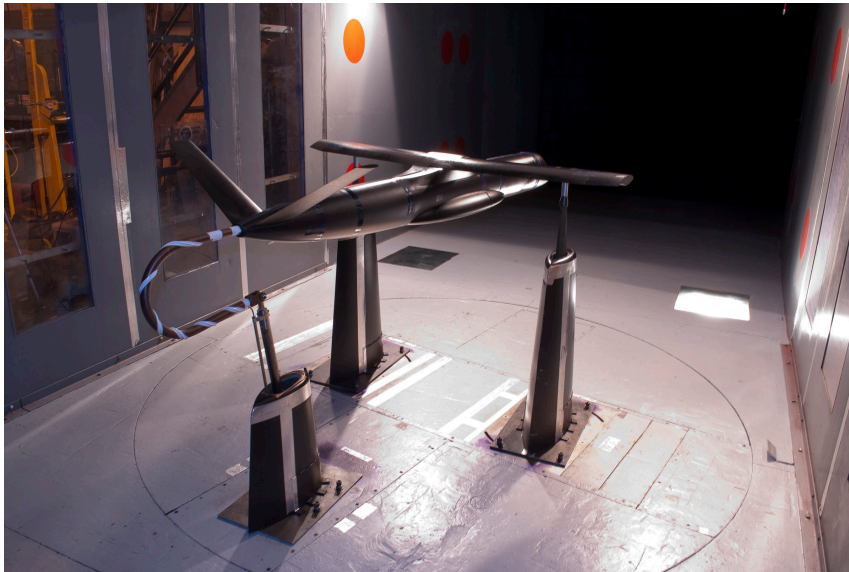
Large Civil Tiltrotor (LCTR) model installed in the Army 7x10-Ft Wind Tunnel at NASA Ames Research Center
