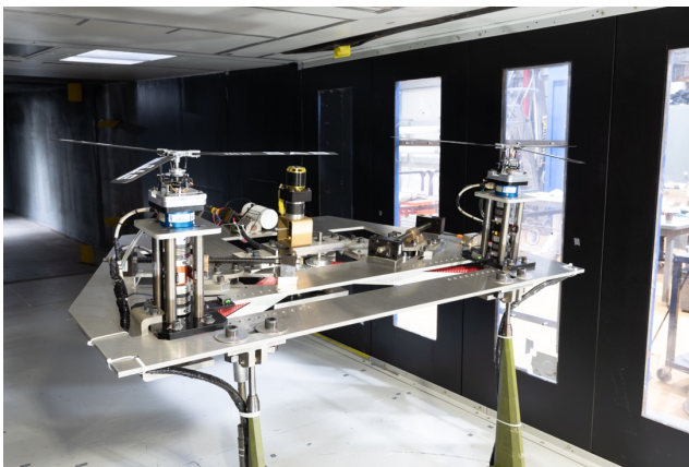
Figure 2. The SBS in the U.S. Army 7- by 10-Foot Wind Tunnel at NASA Ames Research Center
