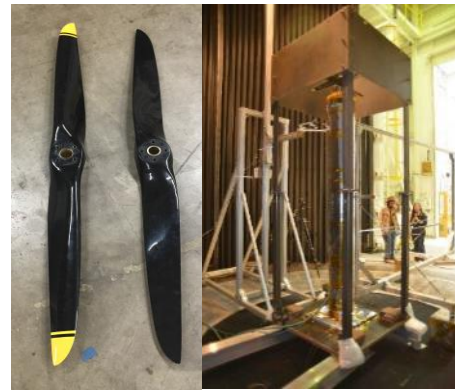
Figure 2. Test propeller and stand setup.
