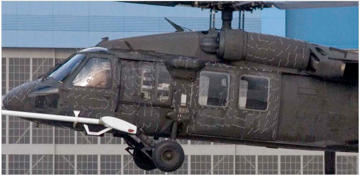
Figure 5(a). Single instantaneous airframe tuft pattern; Wheel height=5 ft.
