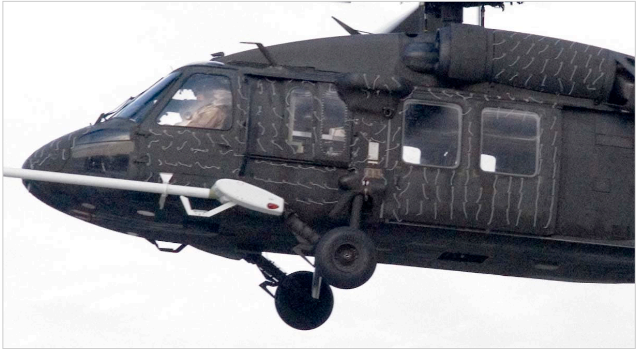
Figure 4(c). Single instantaneous airframe tuft pattern; Wheel height=50 ft.
