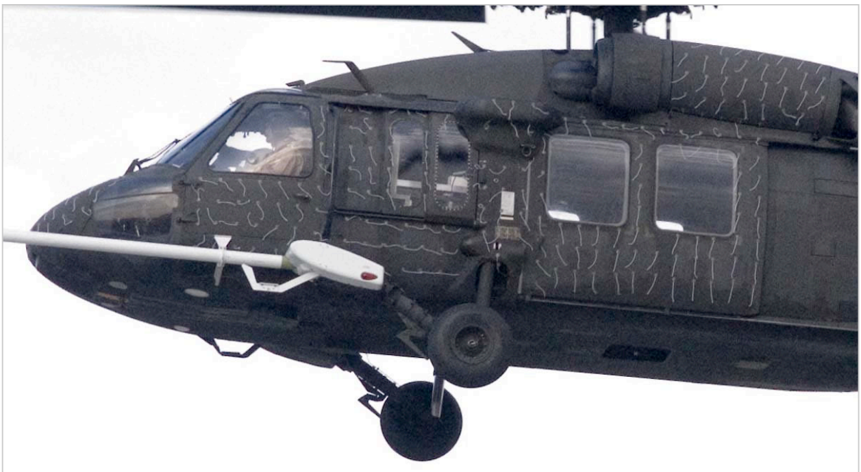
Figure 4(b). Single instantaneous airframe tuft pattern; Wheel height=50 ft.
