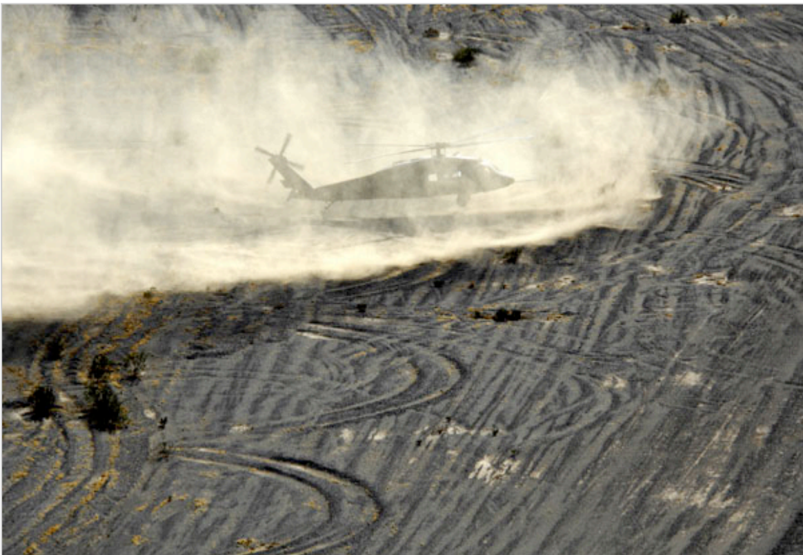
Figure 1. UH-60 Blackhawk performing test landing in brownout at Yuma Proving Grounds.
