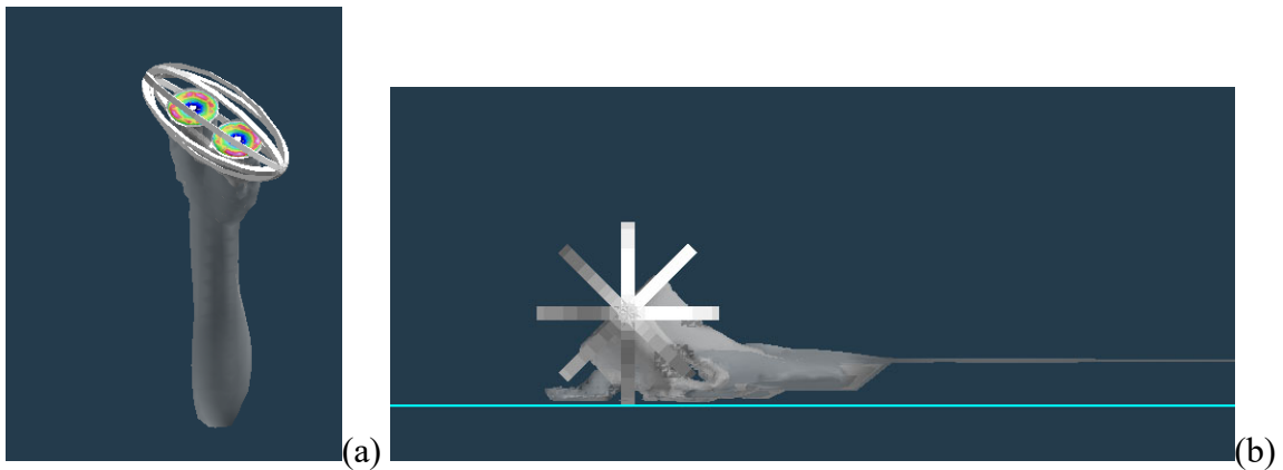
Figure 16. “Pearls” hybrid air/ground mobility robotic system (element) concept: (a) in hover and (b) ground locomotion
