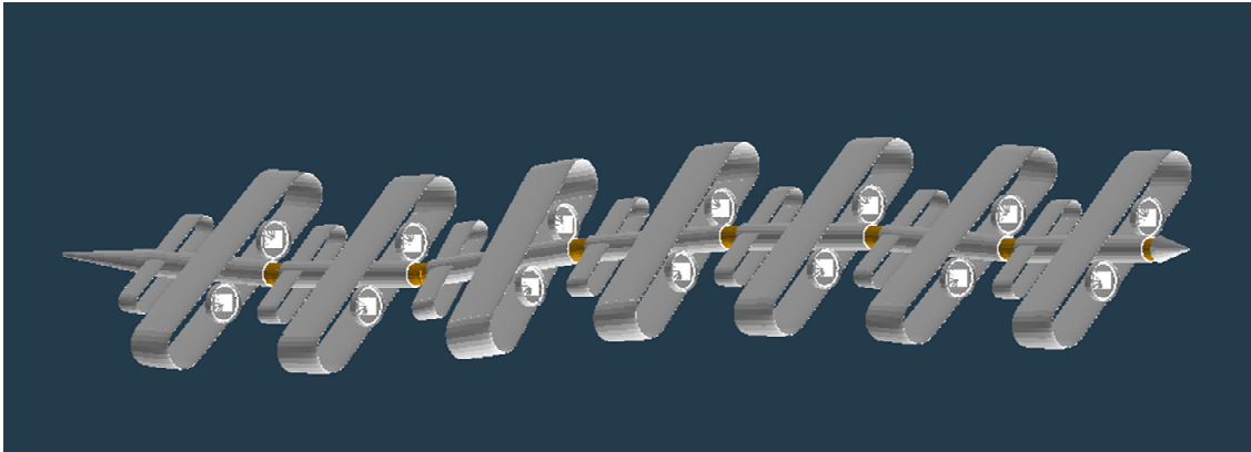
Figure 58. Example of 'fixed' rotor/propeller non-edgewise forward flight ('Skytrain,' Ref. 26)
