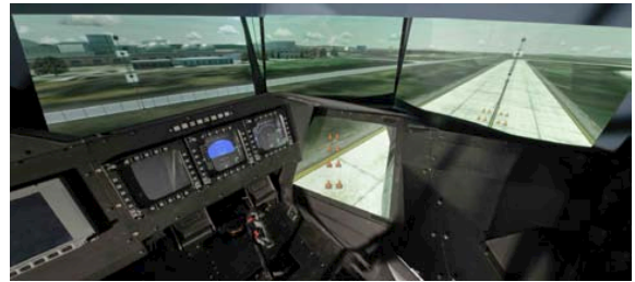
Figure 3. NASA-Ames Vertical Motion Simulator cockpit and displays layout.
