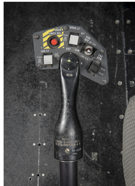
Figure 5. Collective stick inceptor. Note: None of the buttons or switches on the collective inceptor will be used during this experiment.
