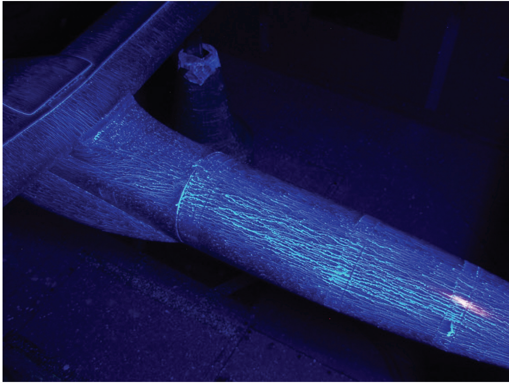
Figure B-83: LS8 flow visualization over fuselage.
