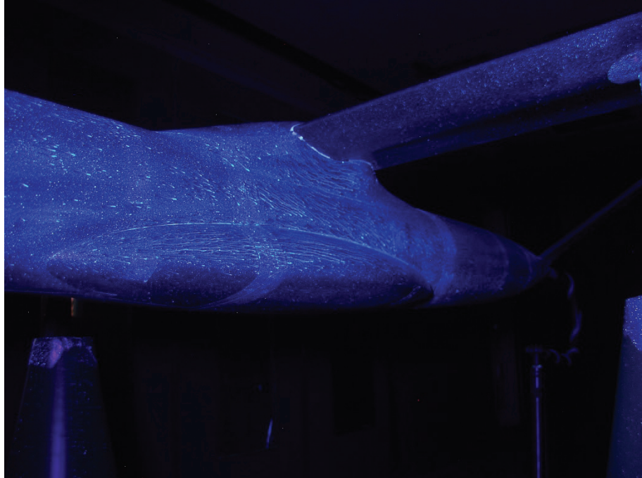
Figure B-37: LSI flow visualization over fuselage and lower wing surface (port).
