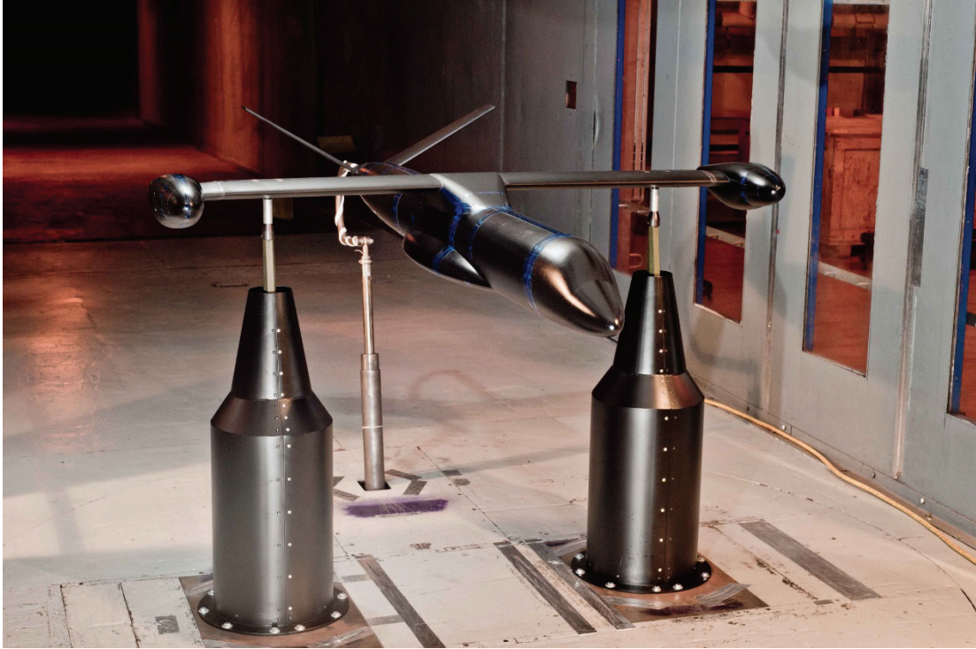
Figure 6: The L00 model configuration mounted inside the wind tunnel with round fairings.
