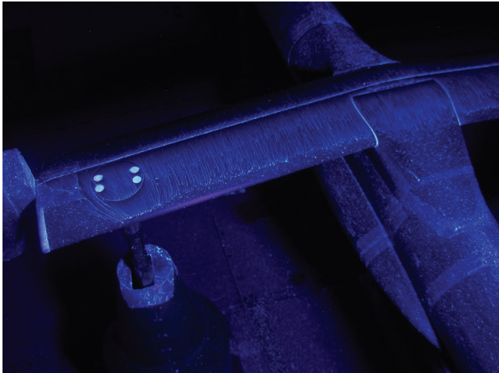
Figure B-84: LS8 flow visualization over wing.
