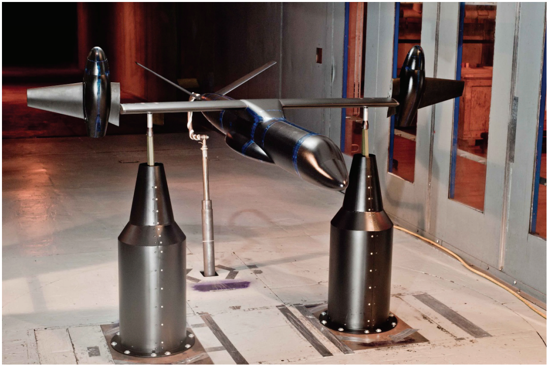
Figure 10: The L75E model configuration mounted inside the wind tunnel with round fairings.
