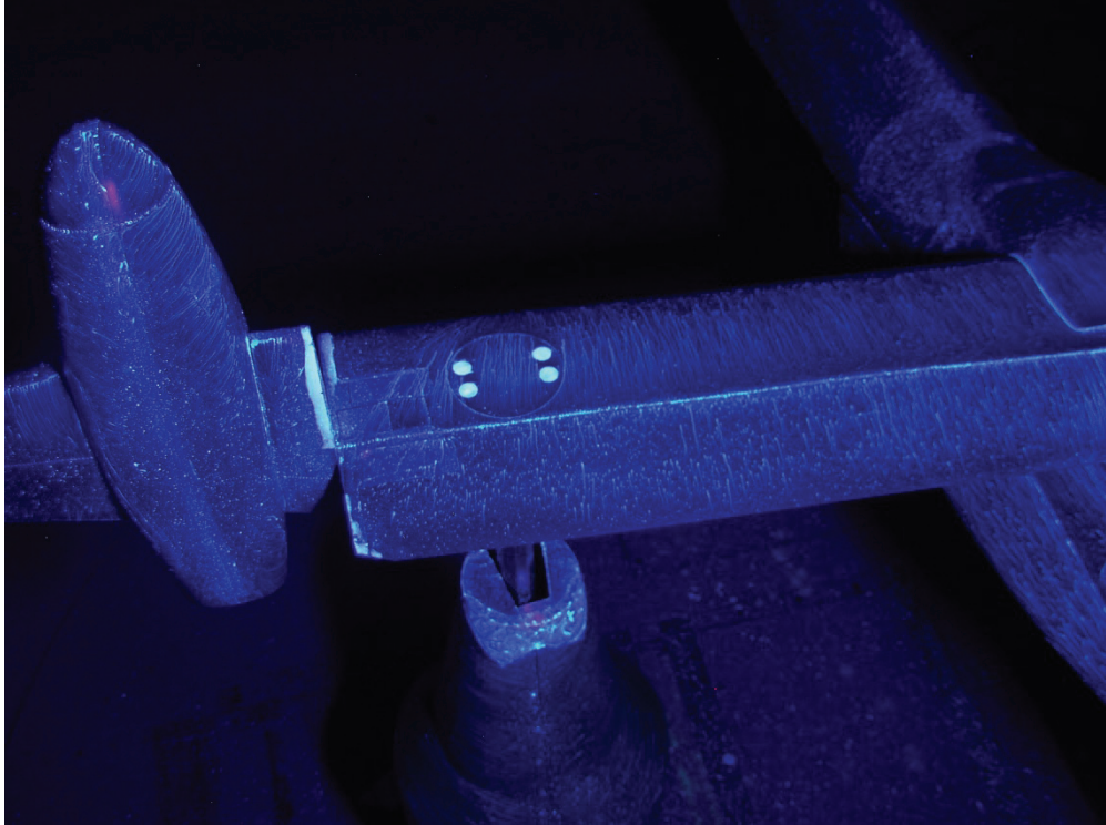
Figure B-85: LS8 flow visualization over nacelle (port-aft).
