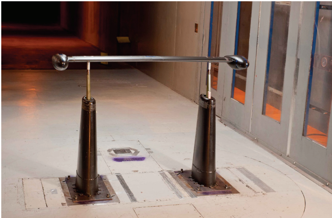
Figure 18: The WN wing-only configuration mounted inside the wind tunnel with aerodynamic fairings.
