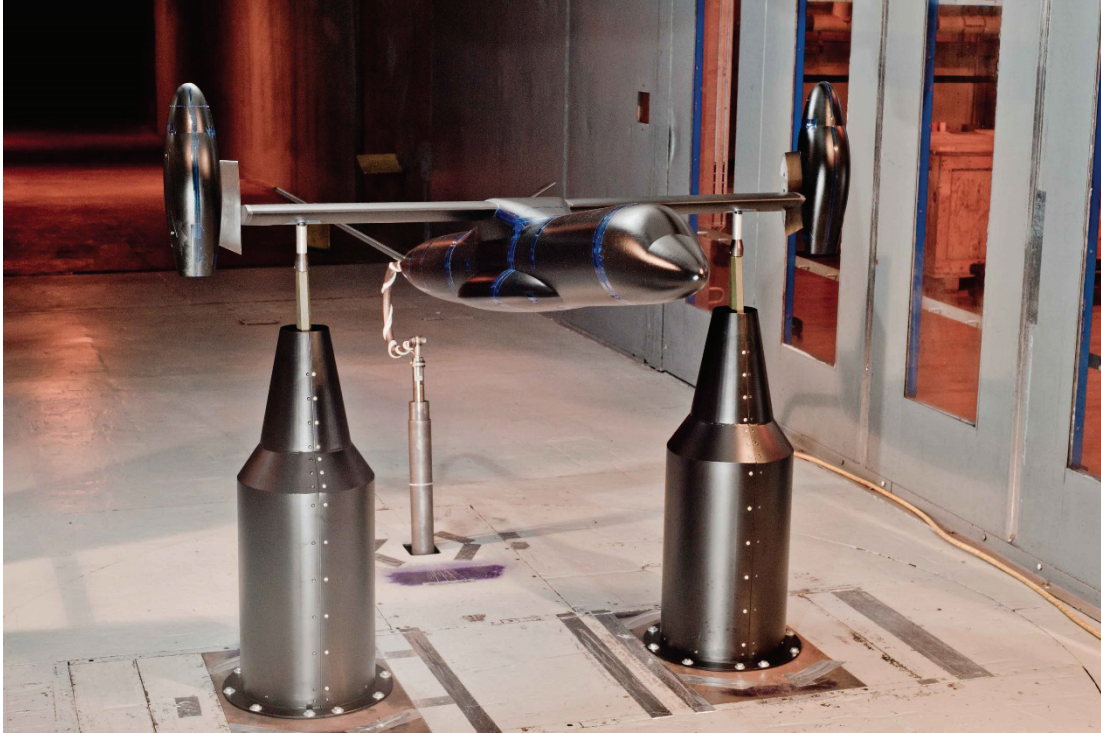
Figure 15: The L85 model configuration mounted inside the wind tunnel with round fairings.
