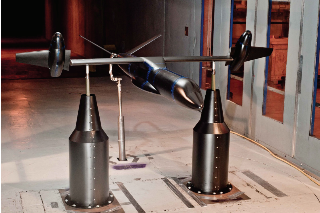
Figure 9: The L60E model configuration mounted inside the wind tunnel with round fairings.
