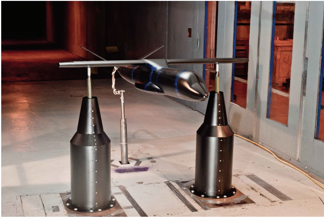
Figure 7: The LNNC model configuration mounted inside the wind tunnel with round fairings.
