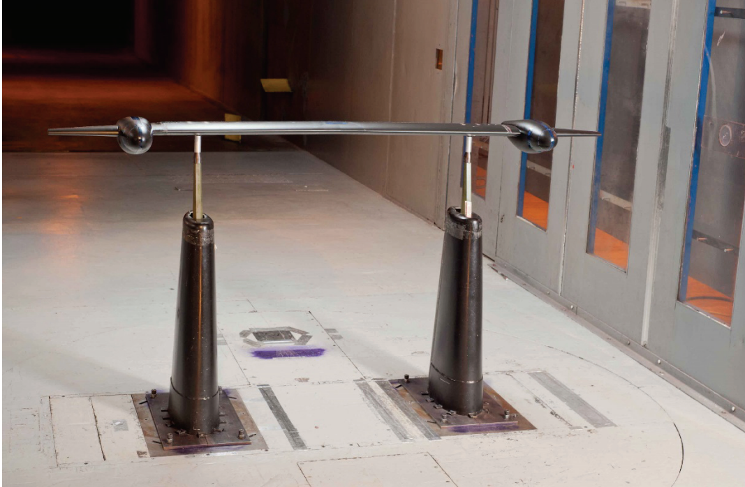
Figure 19: The WNE2L wing-only configuration mounted inside the wind tunnel with aerodynamic fairings.
