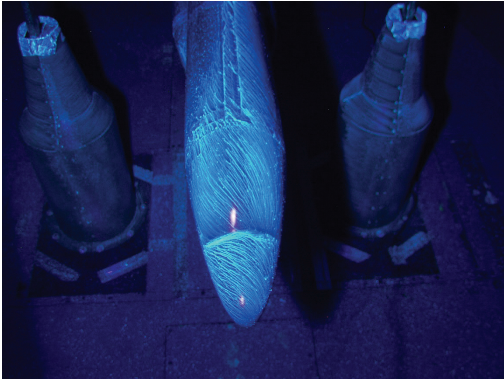
Figure B-115: LS12 flow visualization over nose.
