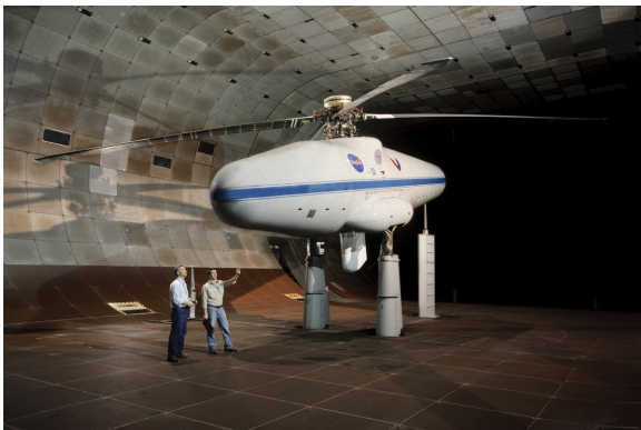
Figure 3: UH-60A rotor system installed in the National Full-Scale Aerodynamics Complex (NFAC) 40- by 80-foot wind tunnel.
