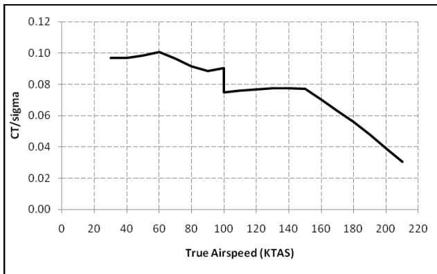
Figure 23. Main rotor C_T/\sigma from velocity sweep
