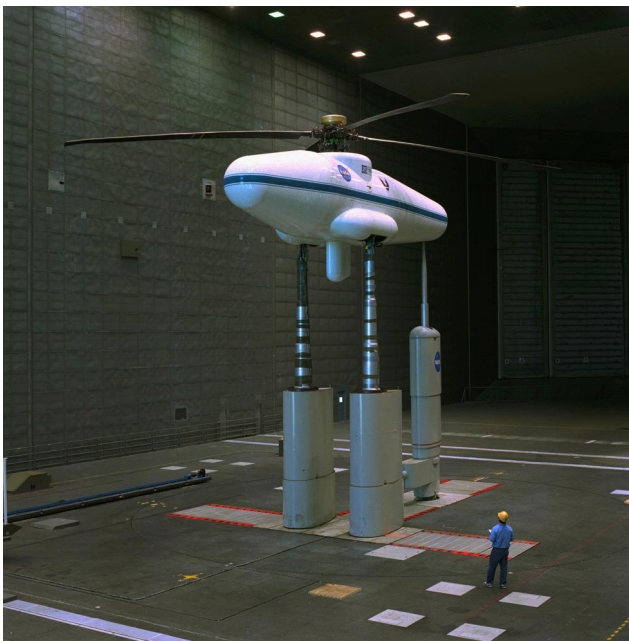
Fig. 1. UH-60 Rotor System installed on Large Rotor Test Apparatus in the Ames 80- by 120-Foot Wind Tunnel.
