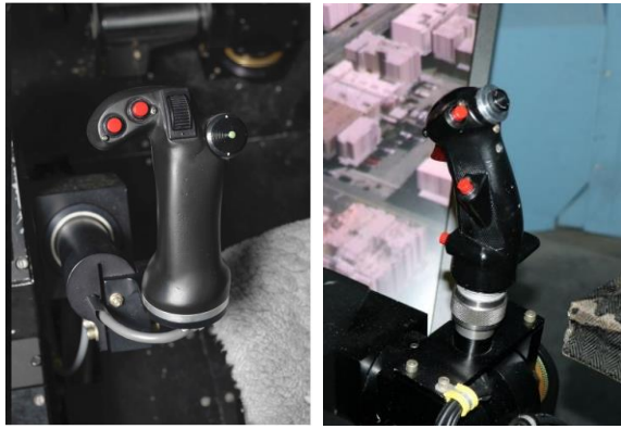
Fig. 5. (Left) Thrust Control Lever (TCL) for vertical control, (Right) Side-stick for pitch and roll control.
