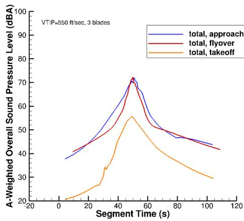
Figure 10b. VTIP=550 ft/sec, 3 blades, 3 flight conditions.
