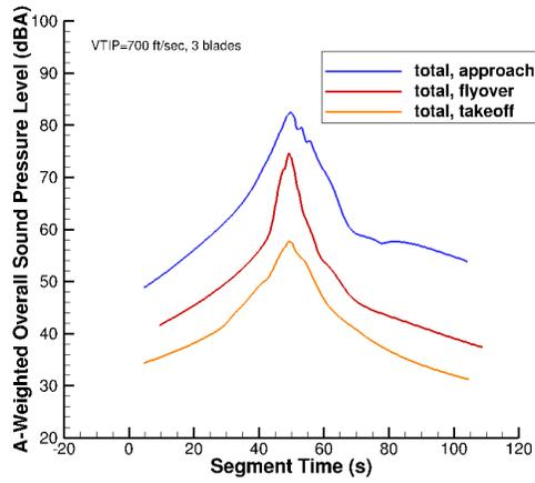
Figure 10a. VTIP=700 ft/sec, 3 blades, 3 flight conditions.
