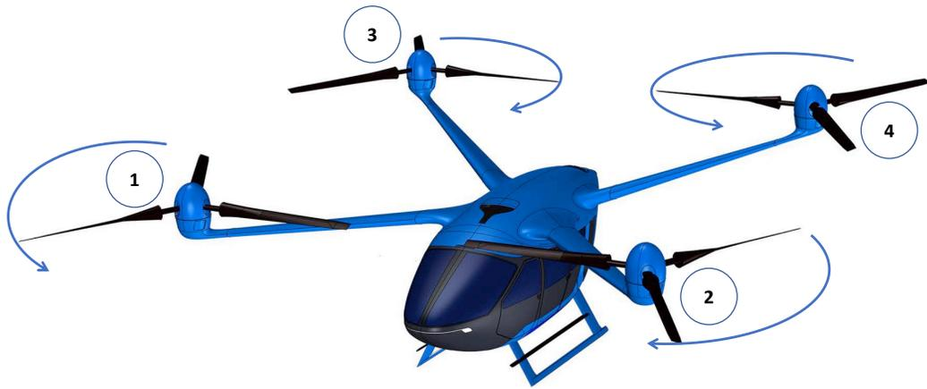
Figure 1b. Quadrotor isometric view, marked with rotor rotation and rotor numbering, Ref. 2.
