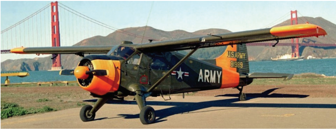
Army L-20A, military version of the civil DHC-2 Beaver short takeoff and landing (STOL) transport.
