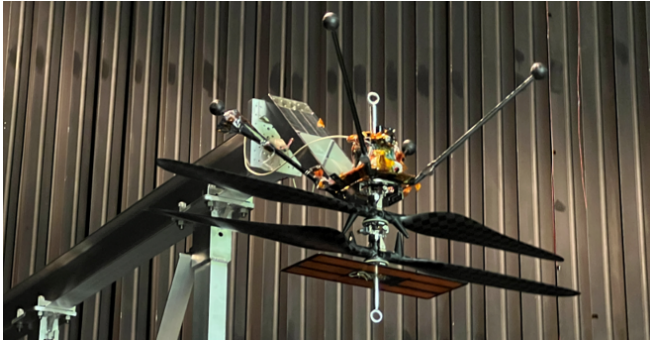
Figure 3. Engineering Design Model 1 (EDM-1) without cruciform box in the 25-foot Space Simulator.
