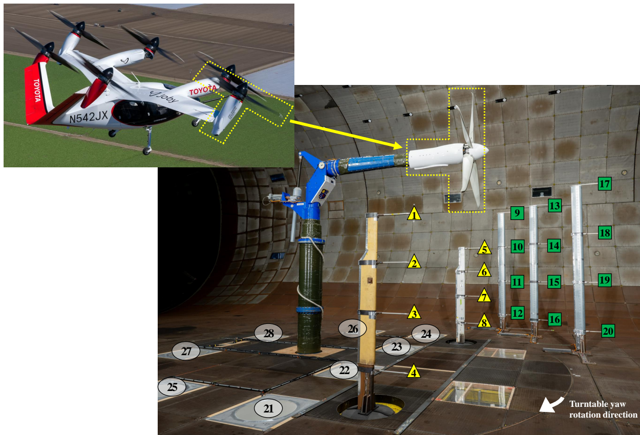
Fig. 2 Joby Aviation Production Prototype S4 aircraft and isolated Joby Aviation aircraft propeller in the NFAC 40- by 80-Foot Wind Tunnel with microphone placement location.
