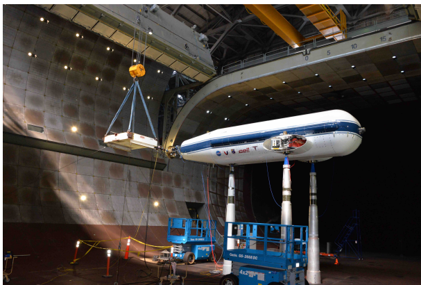
Figure 3. Shake test setup – lateral shaking at hub – 90 deg yaw (helicopter mode)
