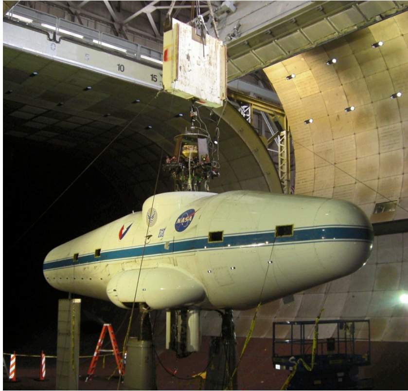
Figure 4. Shake test installation. Vertical shaking on the hub centerline.
