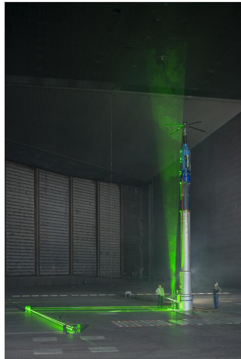
**Figure 1. HVAB rotor mounted in the 80- by 120-ft test section. Laser beam path and sheet expansion for conducting PIV.**
