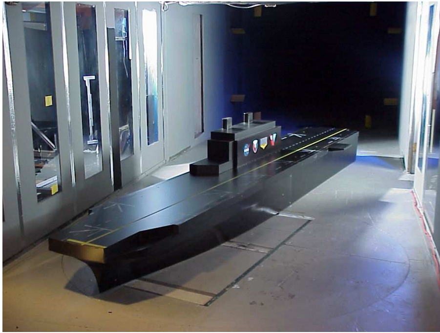
Figure 1. 1/48th-scale amphibious assault ship installed in 7- by 10-Foot Wind Tunnel at NASA Ames.
