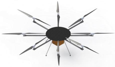
**Figure 20. Octocopter with overlapping blades**
