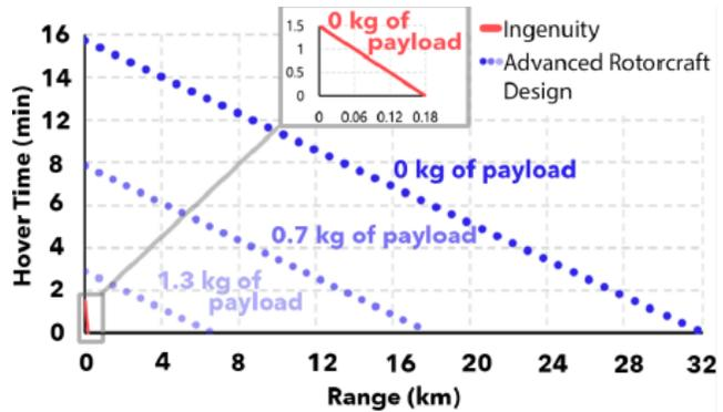
**Figure 7. Mars Science Helicopter concept: 4.6 kg Advanced Mars Helicopter vs. Ingenuity performance (Ref. 32-33)**
