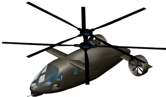
Figure 1. Coaxial Compound Helicopter (CCH) configuration.
