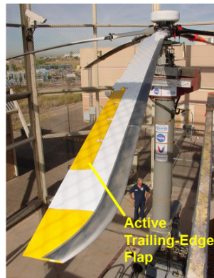
Figure 3. Boeing-SMART rotor with active trailing-edge flap.
