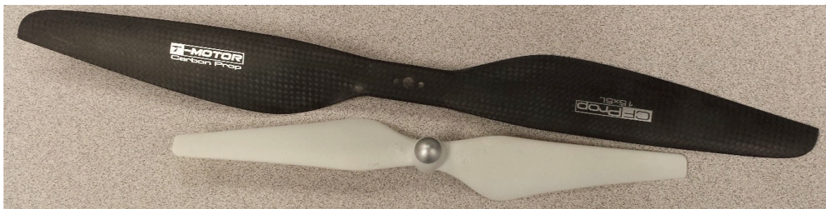
Figure 2: The two types of commercially available quadcopter blades that were studied. The top one is the carbon fiber T-motor 15x5 blade and the bottom one is the DJI Phantom 3 blade.
