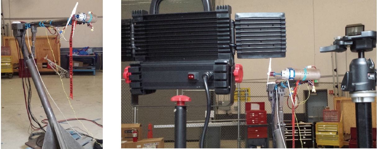
Figure 5: The test setup for the DSLR camera measurements with an isolated rotor fastened to the test stand.
