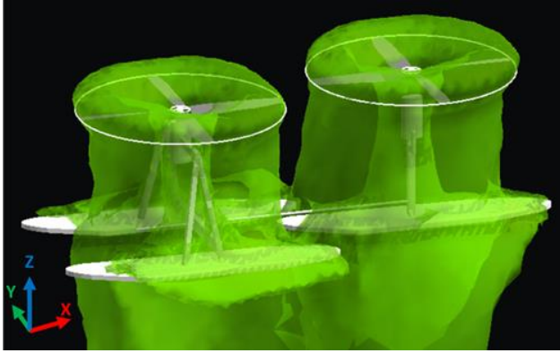
Figure 17. LILI in hover mode: velocity magnitude iso surface flow field prediction ( \theta_{S, \text{front}} = 0^\circ , \theta_{0, \text{front}} = 10^\circ , C_{T, \text{front}} = 0.0253 , \theta_{S, \text{rear}} = 0^\circ , \theta_{0, \text{rear}} = 10^\circ , C_{T, \text{rear}} = 0.0260 ).
