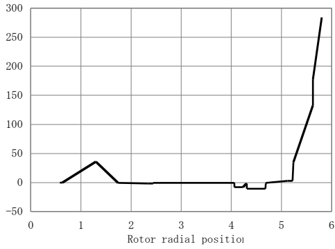
(c) Chordwise CG position, aft of pitch axis (mm).
