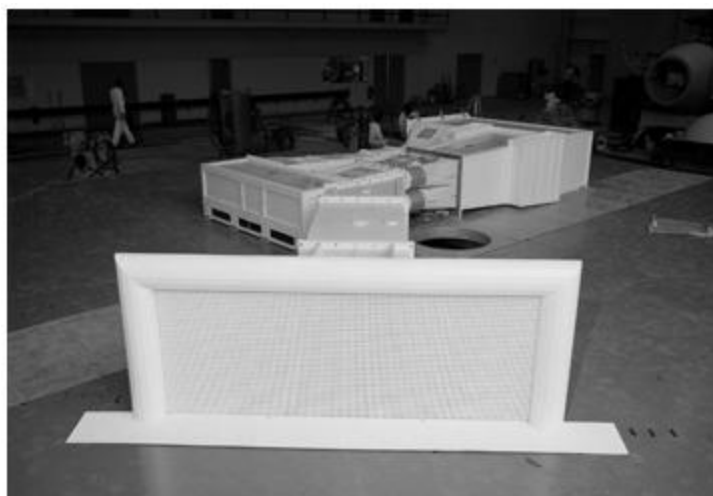
Figure 3. 1/50th-scale model of the NFAC as tested in 1976.
