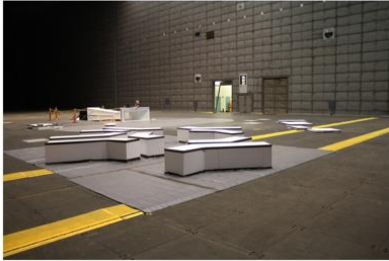
Figure 12. Placement of “Future Blockages” relative to the inlet.
