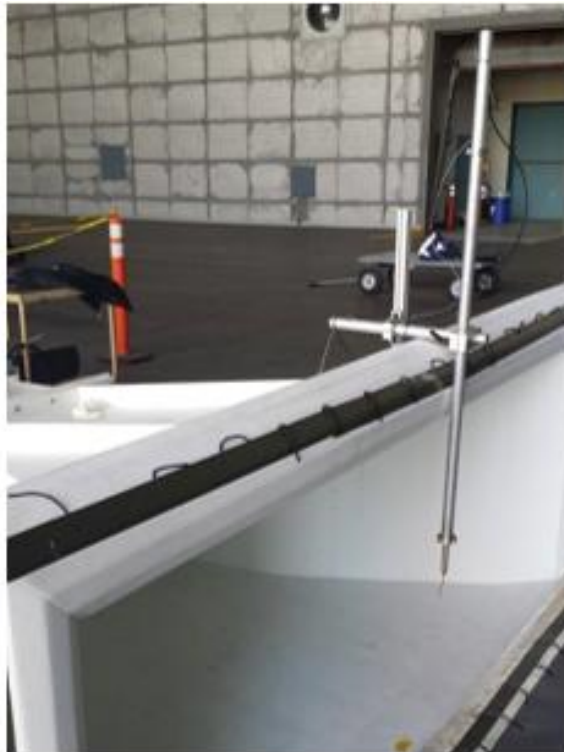
Figure 9. Cobra probe as mounted in the inlet.
