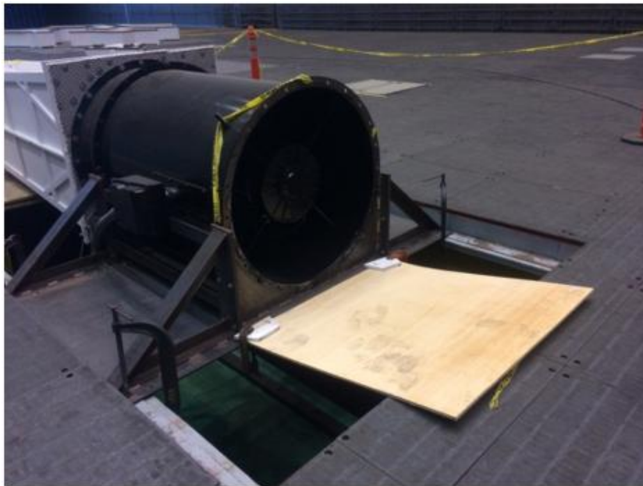
Figure 6. Chicago Blower Co. D/47 vane axial fan attached to the rear of the 1/50th-scale model.
