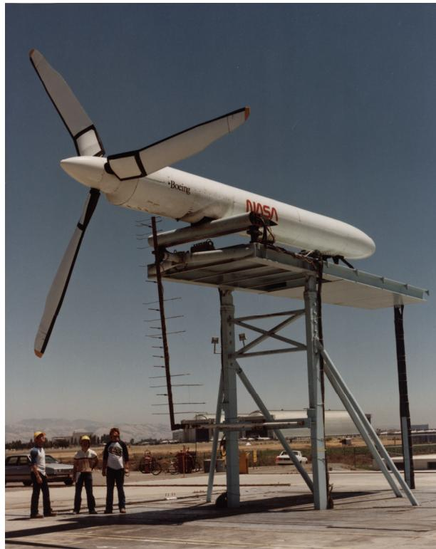
**Figure 8. ATB composite-bladed proprotor tested in hover at the NASA OARF.**
