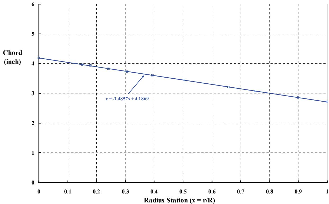
Figure G-3. The 0.15-scale JVX proprotor (four blades)—chord vs. radius station.
