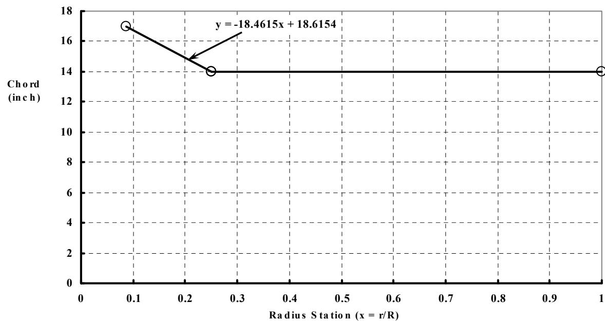
Figure A-3. XV-15 metal-bladed proprotor—chord vs. radius station.
