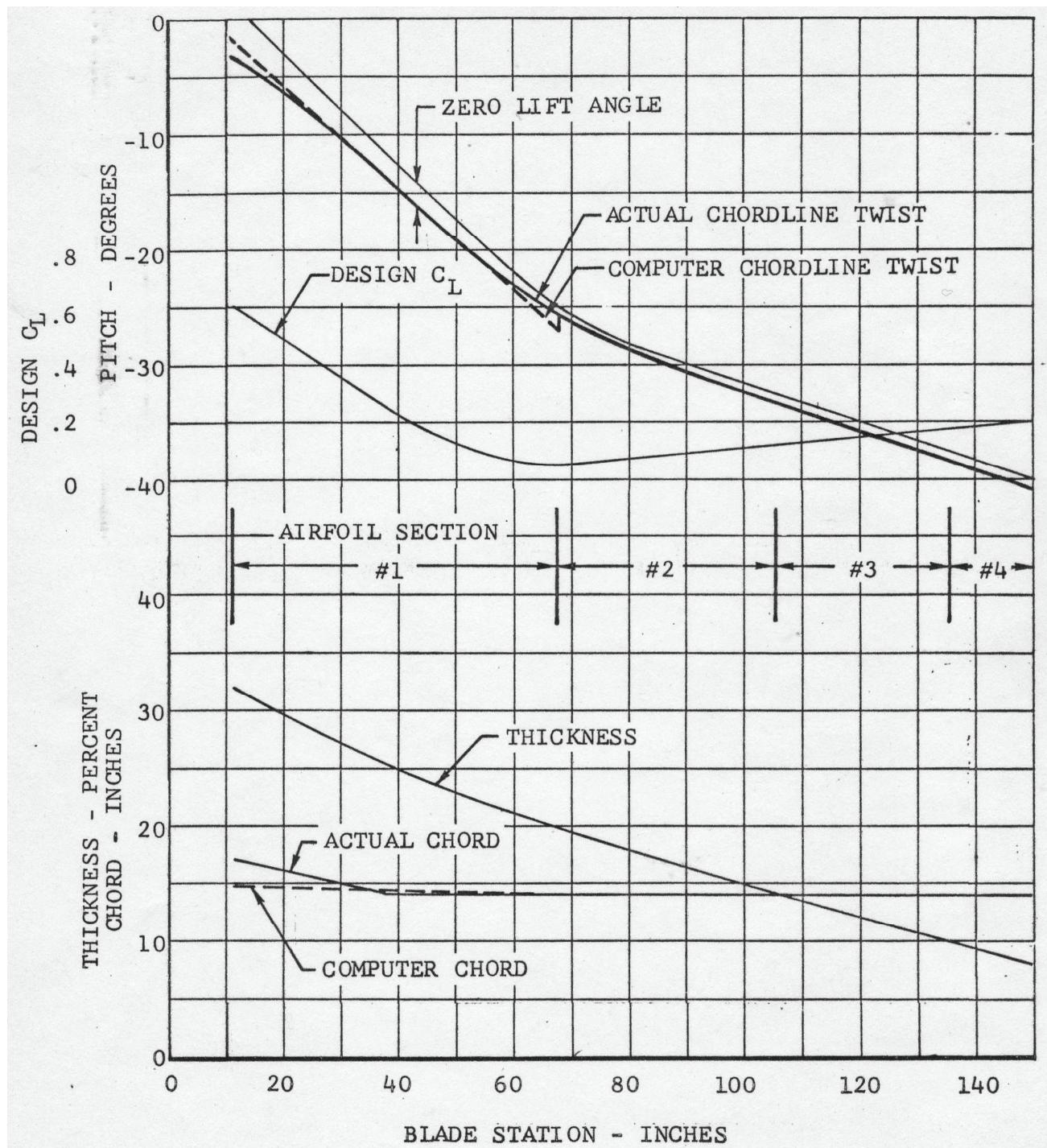
Figure A-1. XV-15 blade geometry. Note: The airfoil sections numbered 1 through 4 only define which airfoil tables of  $C_d$  versus  $C_l$  for several Mach numbers were used in the theory calculations shown in reference 3.
