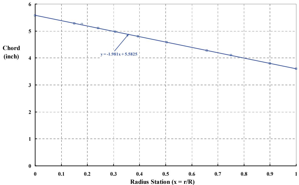
Figure F-3. The 0.15-scale JVX propotor (three blades)—chord vs. radius station.
