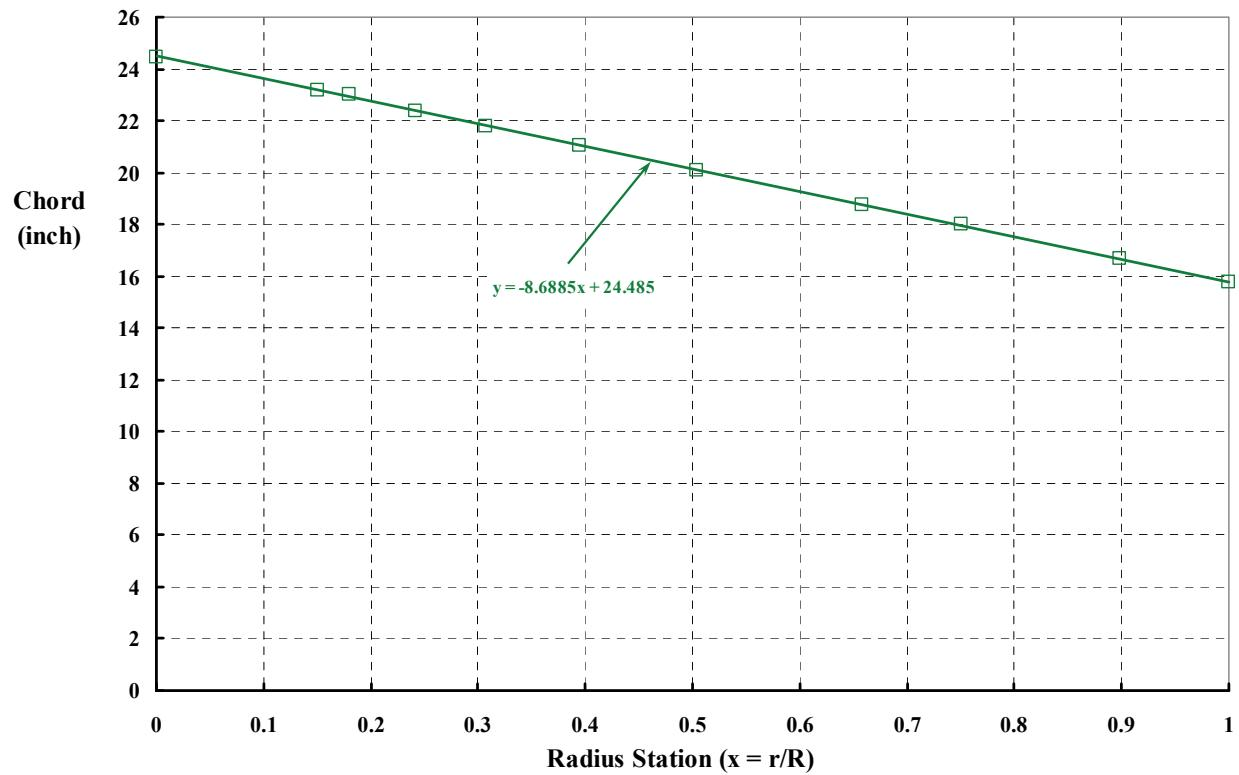
Figure C-3. The 0.658-scale JVX proprotor—chord vs. radius station.
