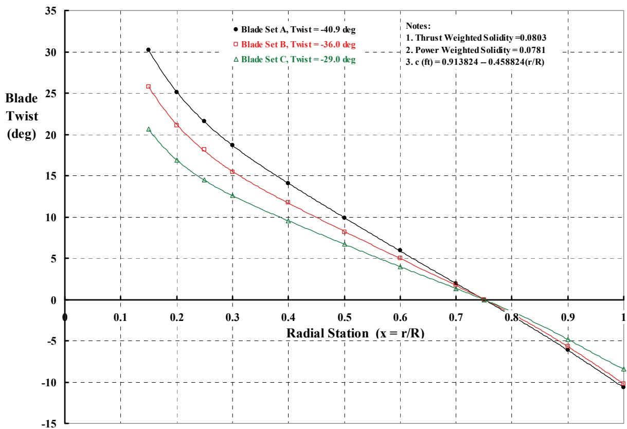
Figure 25. The static twist range of blades tested was from -40 to -29 degrees.
