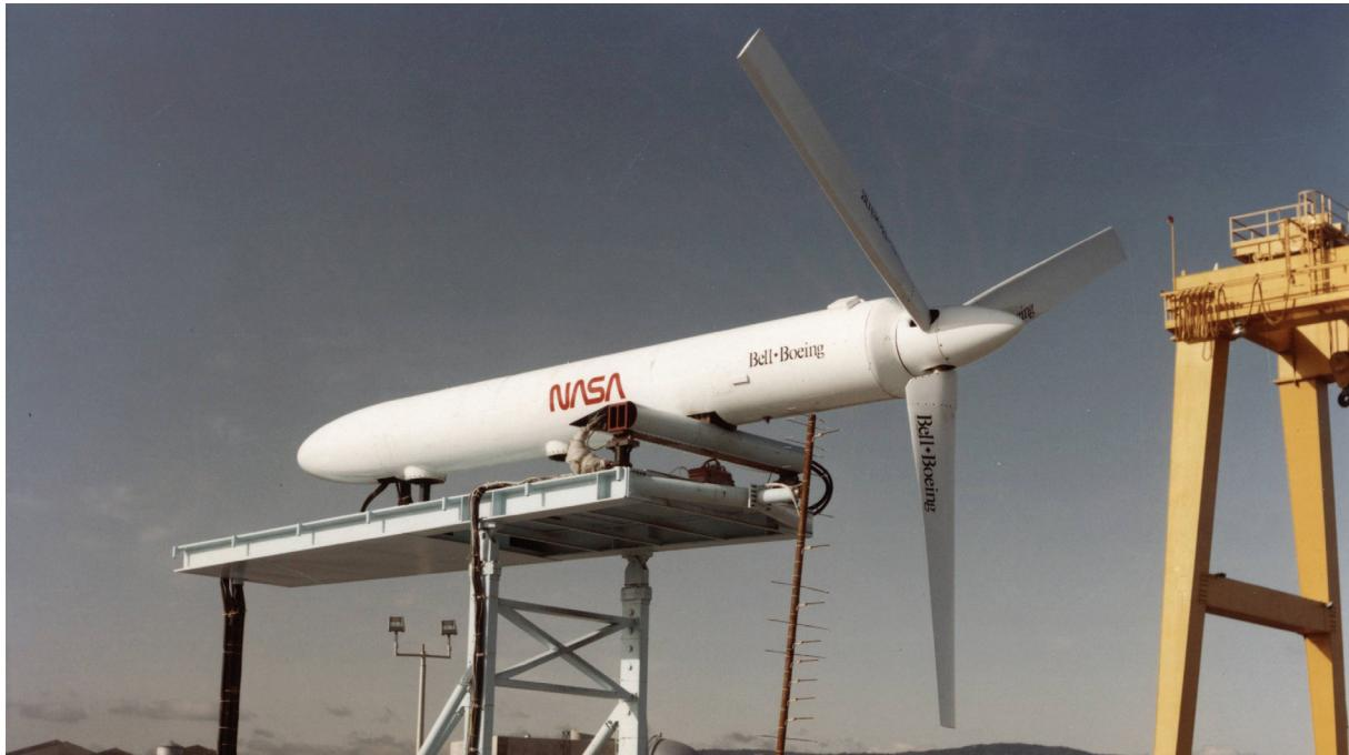
**Figure 10.** The 0.658-scale JVX composite-bladed proprotor tested in hover at the NASA OARF.
