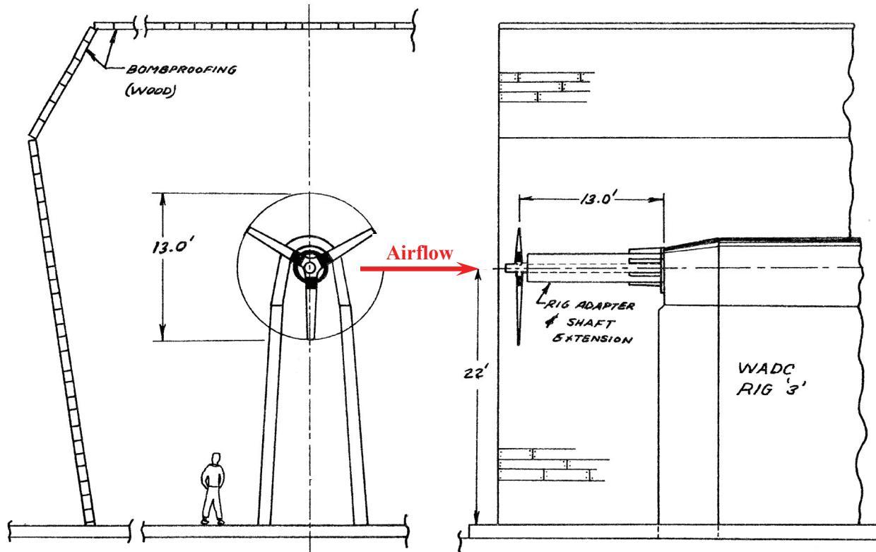
**Figure H-2. WADC Rig #3 had an open face and a standard enclosure to provide safety. Reference 15 discusses tests results with the enclosure removed versus results with the standard enclosure in place.**
