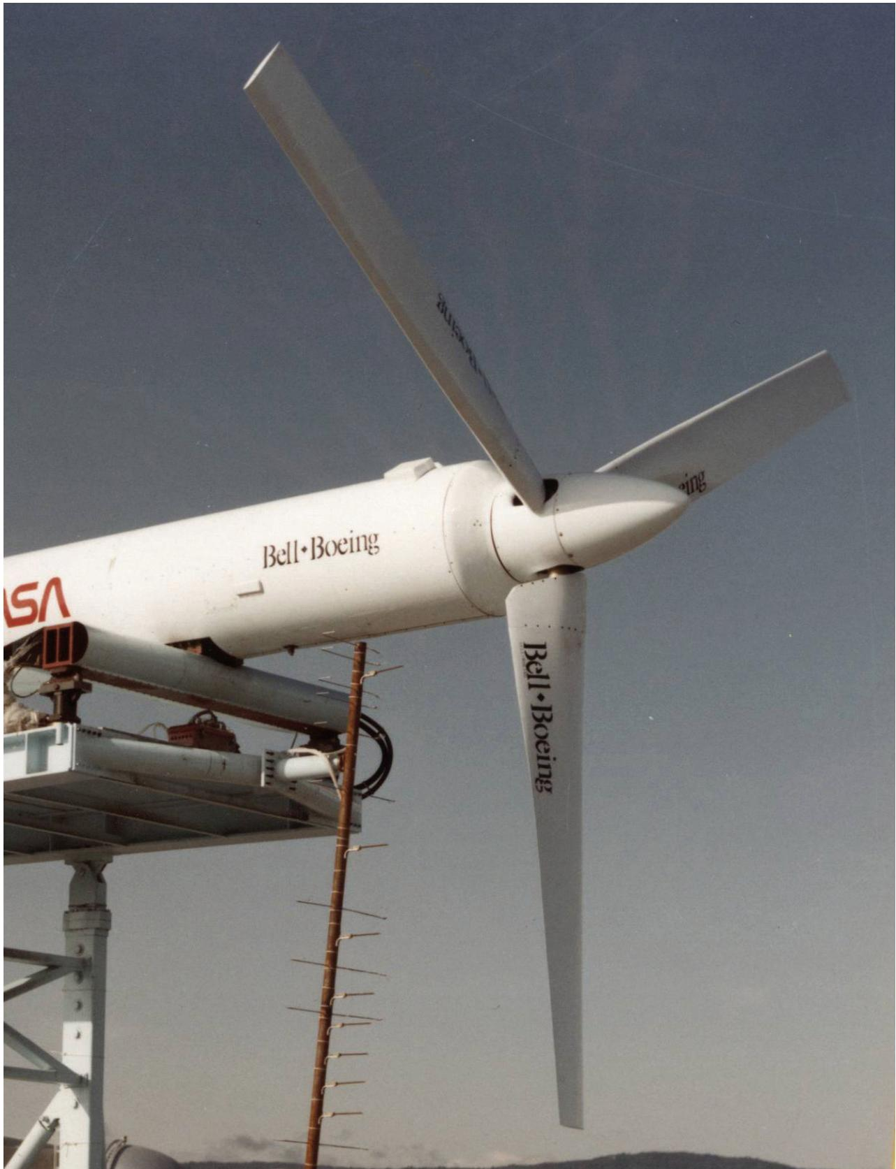
Figure C-1. The 0.658-scale JVX composite-bladed proprotor tested in hover at the NASA OARF.
