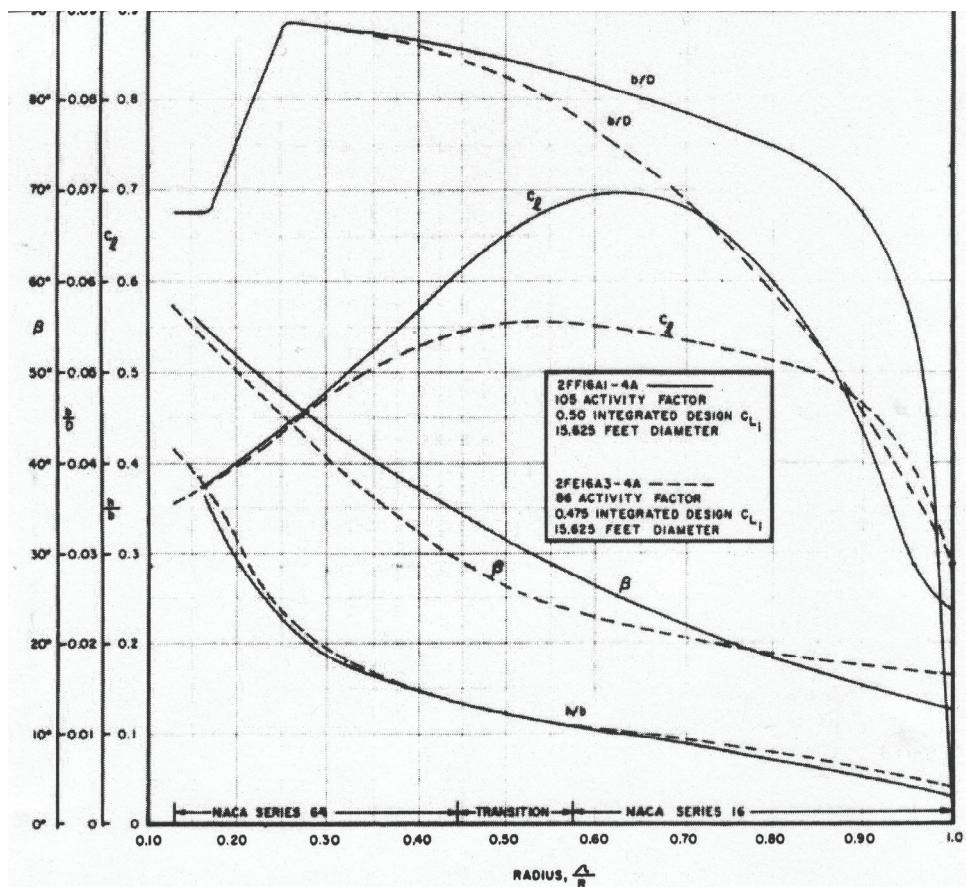
**Figure E-1. Final full-scale propeller (2FF16A1-4A) for the XC-142A. Follow the solid lines.
