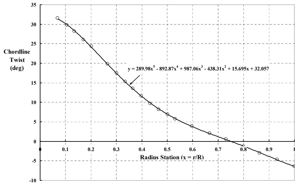
Figure A-2. XV-15 metal-bladed proprotor—twist vs. radius station.
