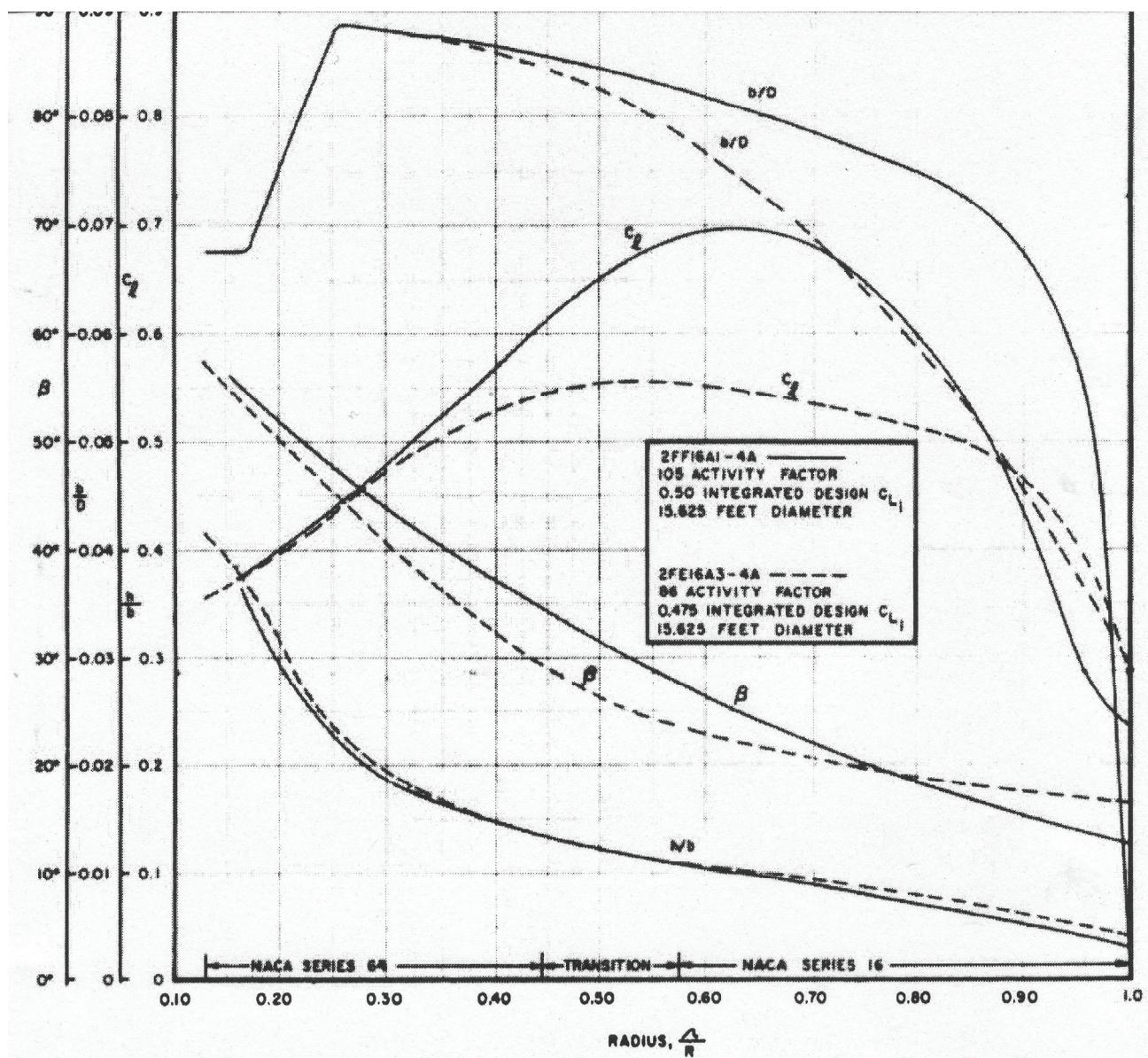
Figure D-3. Initial full-scale propeller (2FE16A3-4A) for the XC-142A. Follow the dashed lines.
