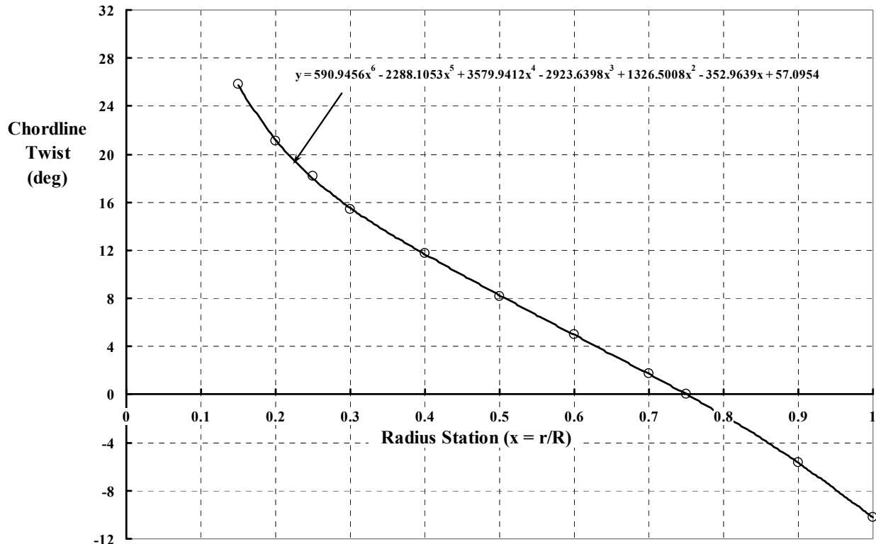
Figure I-1. The 0.2364-scale Proprotor B for Boeing Vertol Model 160—twist vs. radius station.
