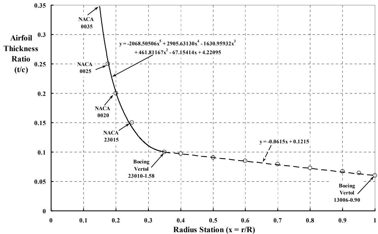
**Figure H-5.** The 0.2364-scale Proprotor A for Boeing Vertol Model 160—airfoil thickness ratio vs. radius station. The Boeing Vertol 23010-1.58 is a NACA 23010 with increased nose radius. The Boeing Vertol 13006-0.90 is a NACA 13006 with increased nose radius.
