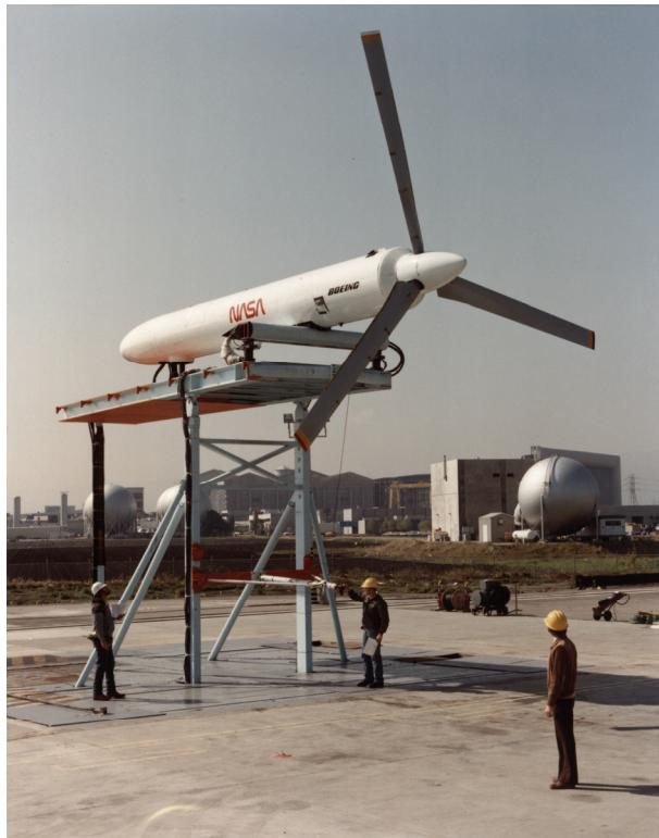
**Figure 7. XV-15 metal-bladed proprotor tested in hover at the NASA OARF.**
