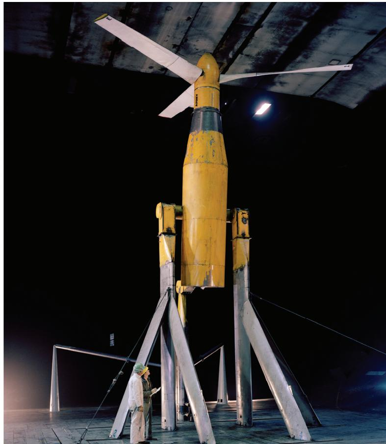
**Figure 5.** XV-15 metal-bladed proprotor tested in hover in the NASA Ames 40- by 80-foot wind tunnel.
