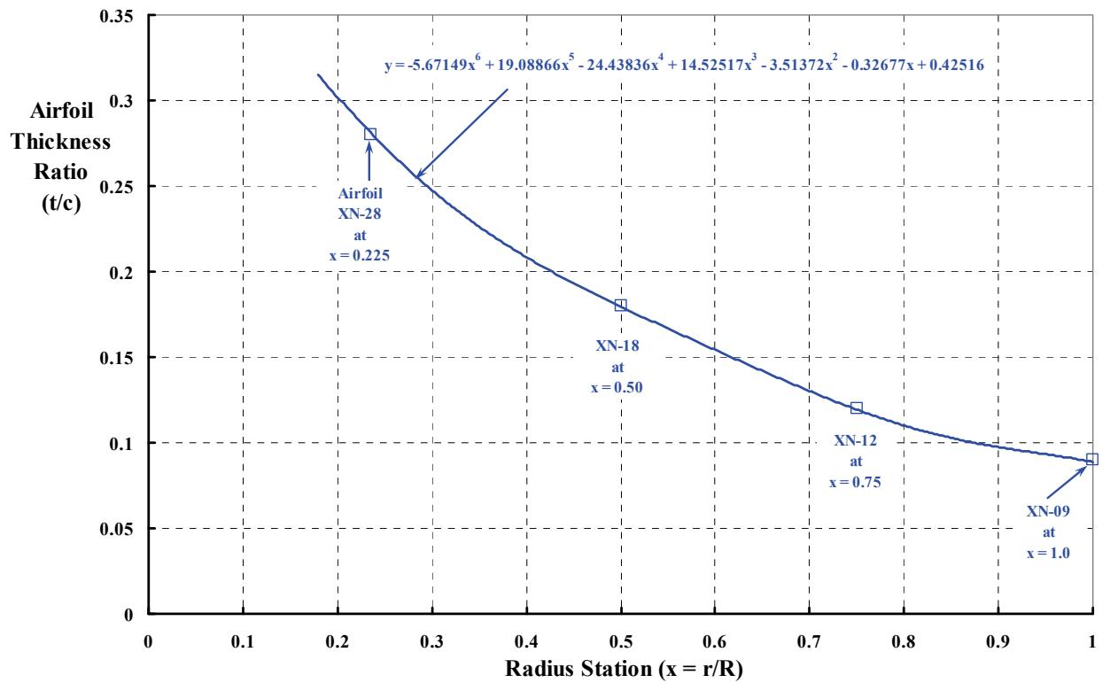
Figure F-4. The 0.15-scale JVX propotor (three blades)—airfoil thickness ratio vs. radius station.
