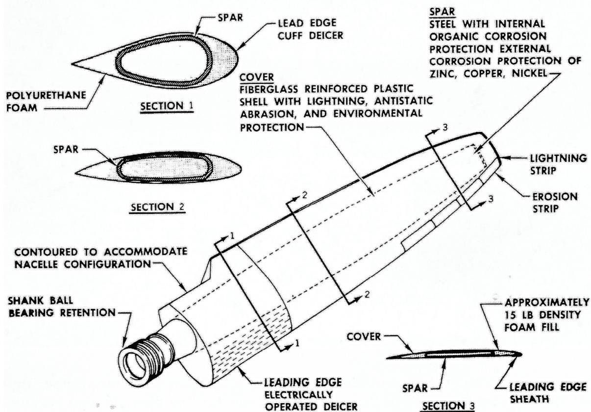
Figure 11. XC-142A blade assembly features.
