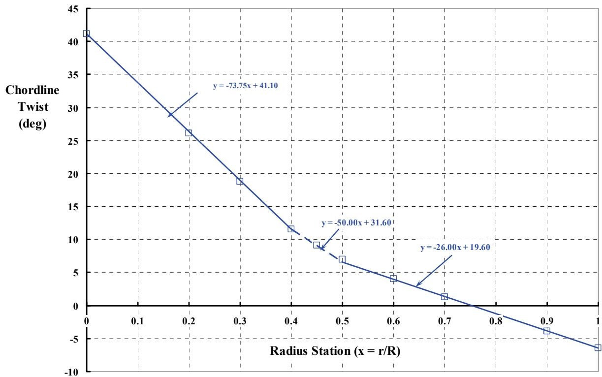
Figure F-2. The 0.15-scale JVX propotor (three blades)—twist vs. radius station.
