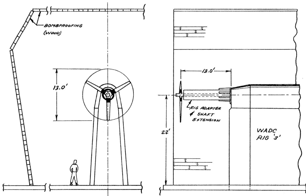
Figure 27. WADC Rig #3 propeller test stand with 13-foot shaft extension.
