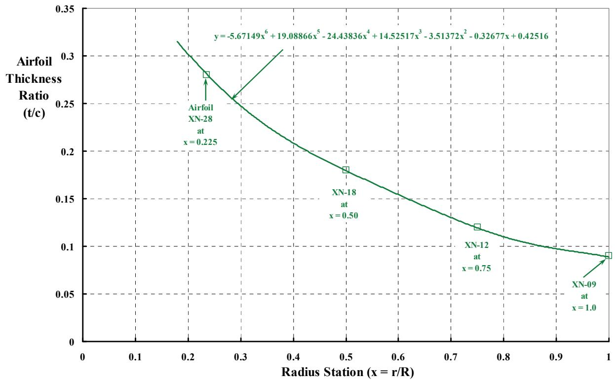
Figure C-4. The 0.658-scale JVX propotor—airfoil thickness ratio vs. radius station.
