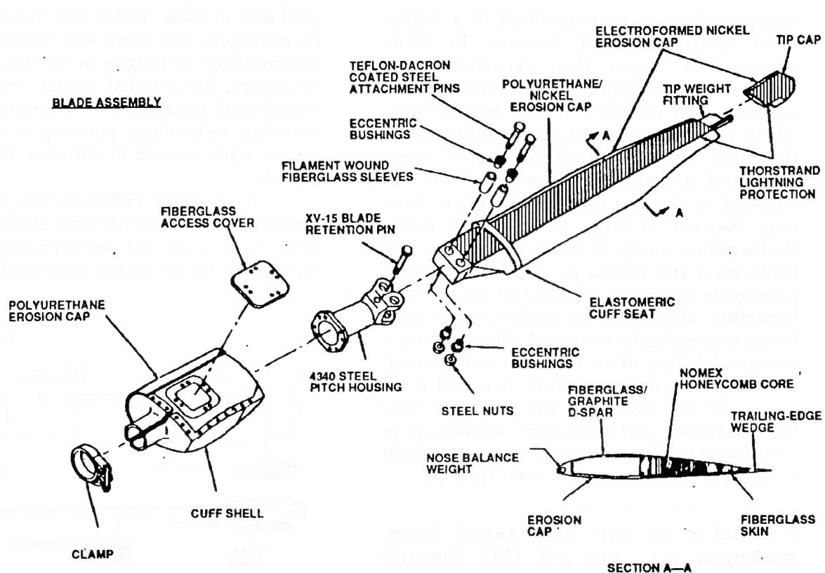
**Figure 9. ATB assembly features.**
