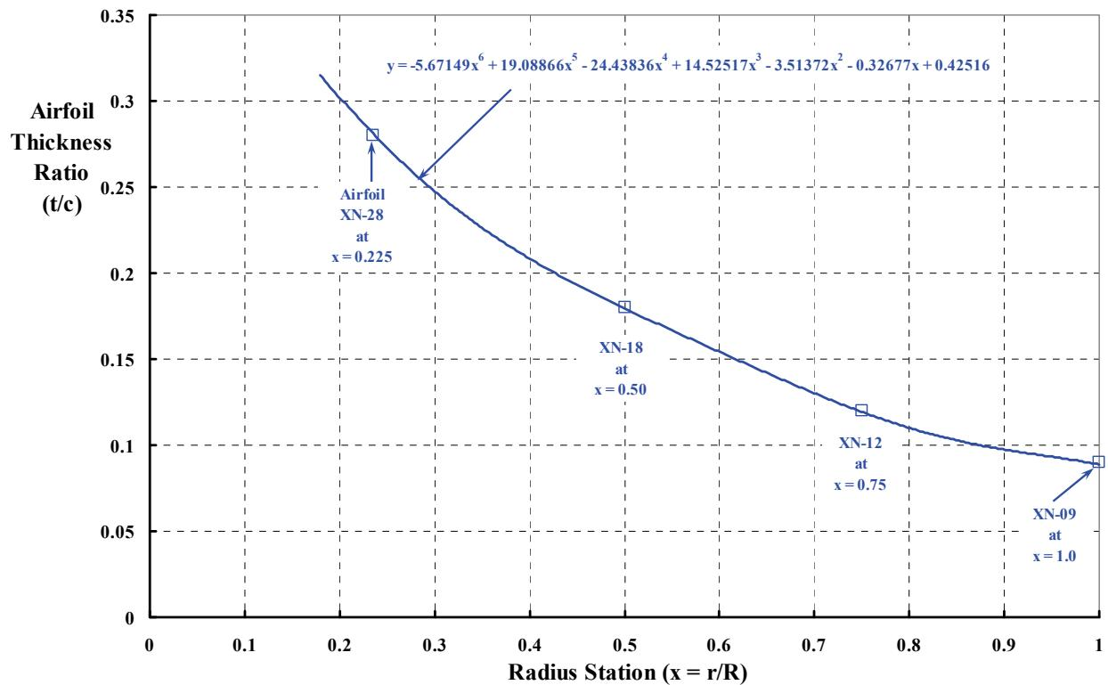
Figure G-4. The 0.15-scale JVX propotor (four blades)—airfoil thickness ratio vs. radius station.
