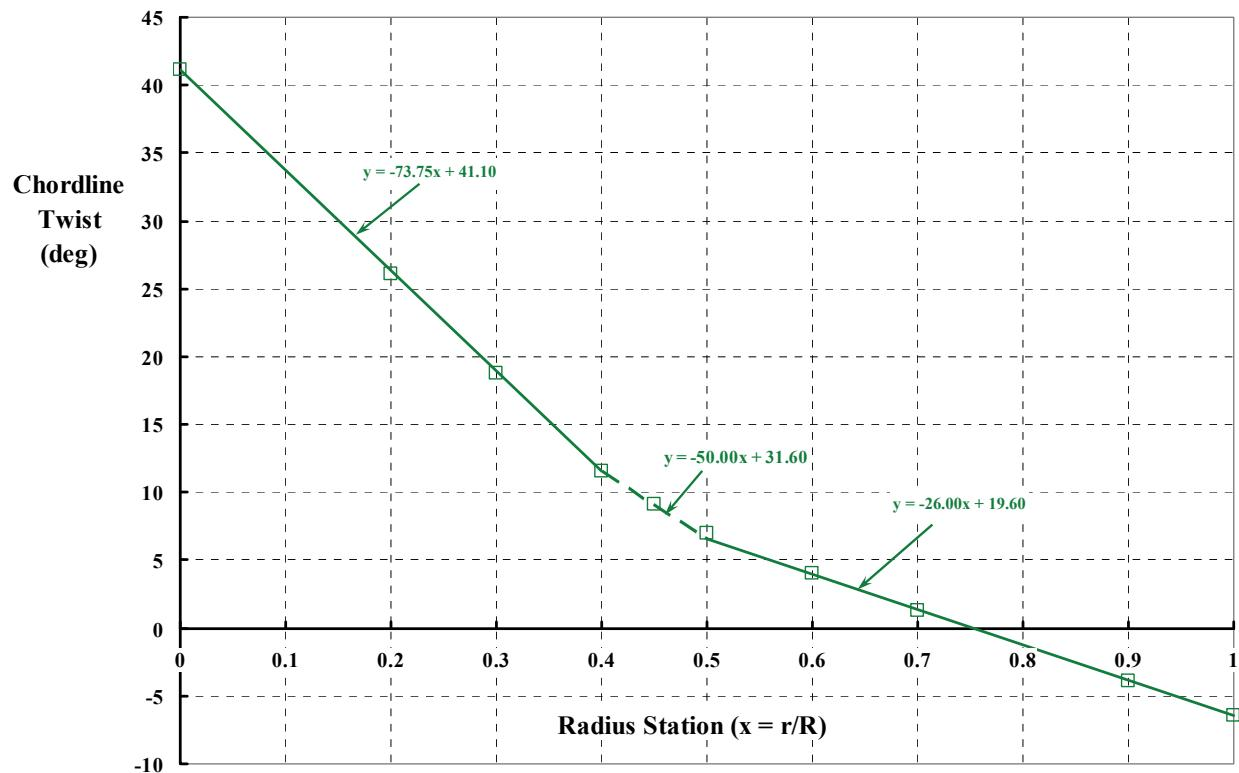
Figure C-2. The 0.658-scale JVX proprotor—twist vs. radius station.
