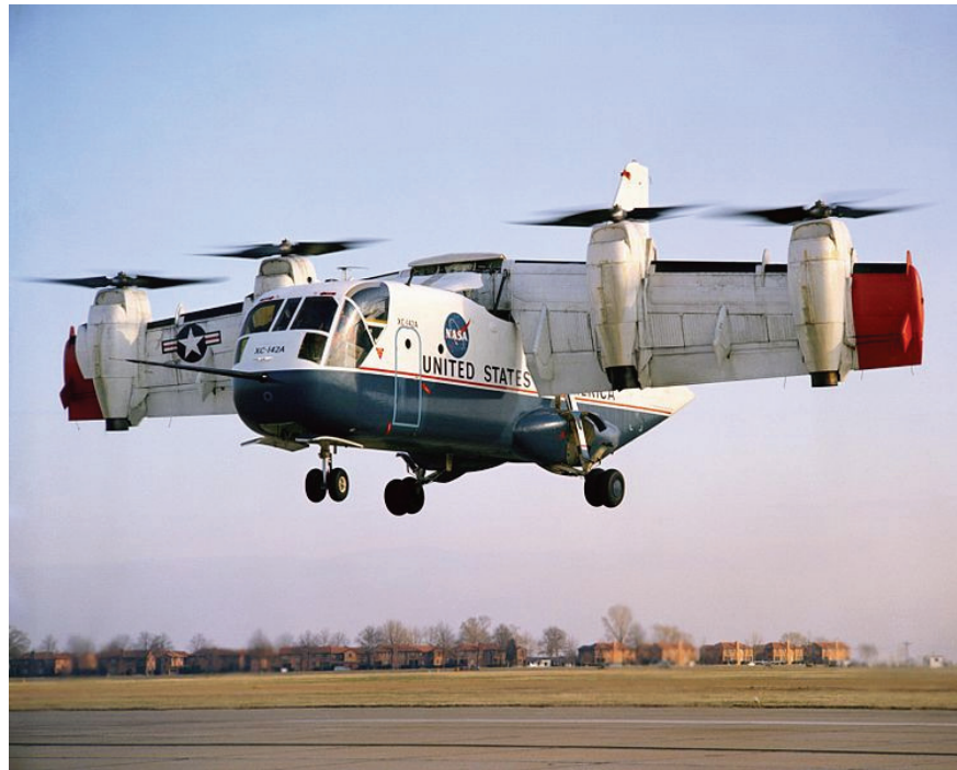
Figure 1. The XC-142A tiltwing was built by Ling-Temco-Vought and Hiller and Ryan after they won the U.S. Air Force Tri-Service competition for an assault transport. The 41,500-pound aircraft, with a weight empty of 24,700 pounds, first flew on September 29, 1964. The initial design gross weight was 37,474 pounds.
