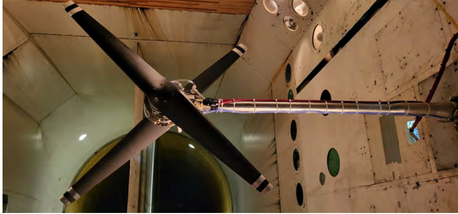
Fig. 7 Flight-like Dragonfly coaxial rotor system installed in the TDT. The depicted coaxial rotor orientation is for a vertical or near-vertical climb condition ( \alpha \approx -90 deg). Image courtesy of the Dragonfly TDT Test Team.
