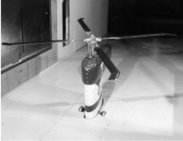
Fig. 2 Swept-tip rotor on RTR test stand in the Army/NASA 7- by 10-Foot Wind Tunnel.
