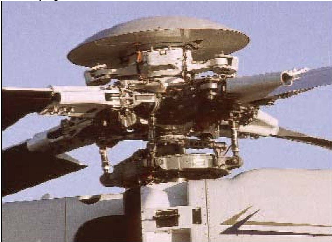
Figure 15a. Sikorsky S-92 hub and rotating controls in detail.
