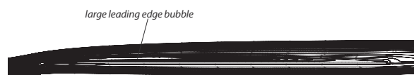
Figure 19. Streamlines for the flat plate showing a steady bubble ( \alpha = 5.0^\circ , M = 0.20 , Re_c \approx 2.0 \cdot 10^3 )
