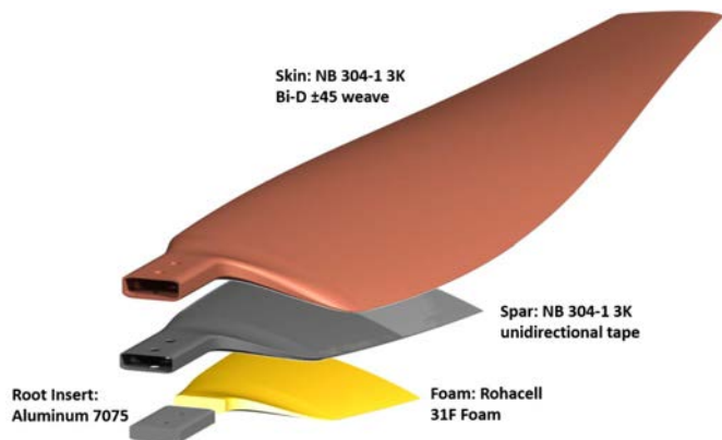
Fig. 24. Materials and internal structure of the ROAMX blade (from Ref. 4).
