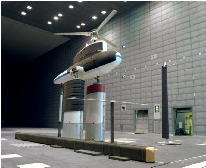
Fig 1. XV-15 right-hand rotor mounted on the RTA in the NASA Ames 80- by 120-Foot Wind Tunnel.
